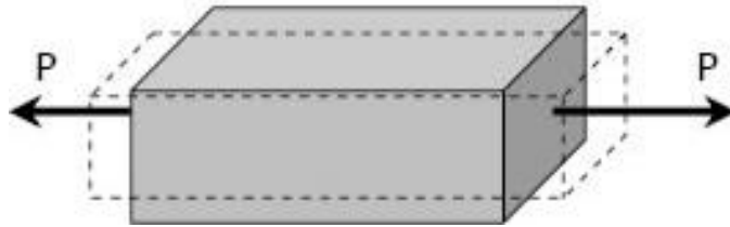
Fig. 3.1 Schematic diagram of the lateral contraction effect of a material due to the application of a normal force, which is determined by the Poisson's ratio.
