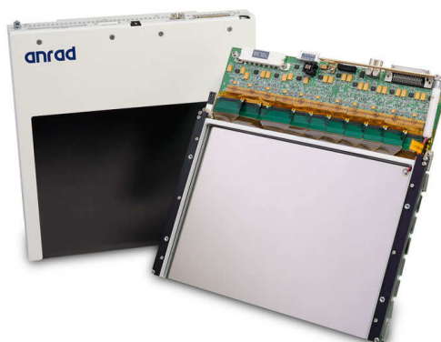
Figure 1.1: Anrad SMAM DCXID for digital mammography (Figure from www.anrad.com ).
