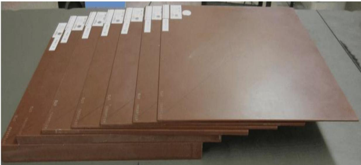
Figure 2.5: Slabs of CTG Gammex Model 457 solid water phantom.
