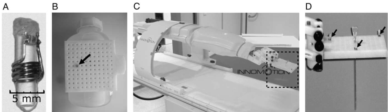
Fig. 1. (A) MR-visible marker consisting of a small solenoid RF coil (outer diameter 4.6 mm, length 4 mm) and a ceramic chip capacitor. (B) Setup for accuracy measurements showing marker board (12×12×2 cm) and phantom bottle (diameter 12 cm, length 25 cm). One ICRF marker (arrow) was scanned five times in each of the 44 accurately defined positions along the x - and z -direction. (C) Robotic manipulator (Innomotion) with six degrees of freedom mounted on the patient table. Different instruments can be attached to a so-called application module (AMO) at the end of the robotic arm. (D) Custom-made board [dotted frame in (C)] with three MR-visible markers (arrows) and model instrument (16G coaxial needle, 150 mm long; Invivo, Schwerin, Germany) attached to the AMO. The needle is inserted at the position of the marker centroid and aligned perpendicular to the board.
