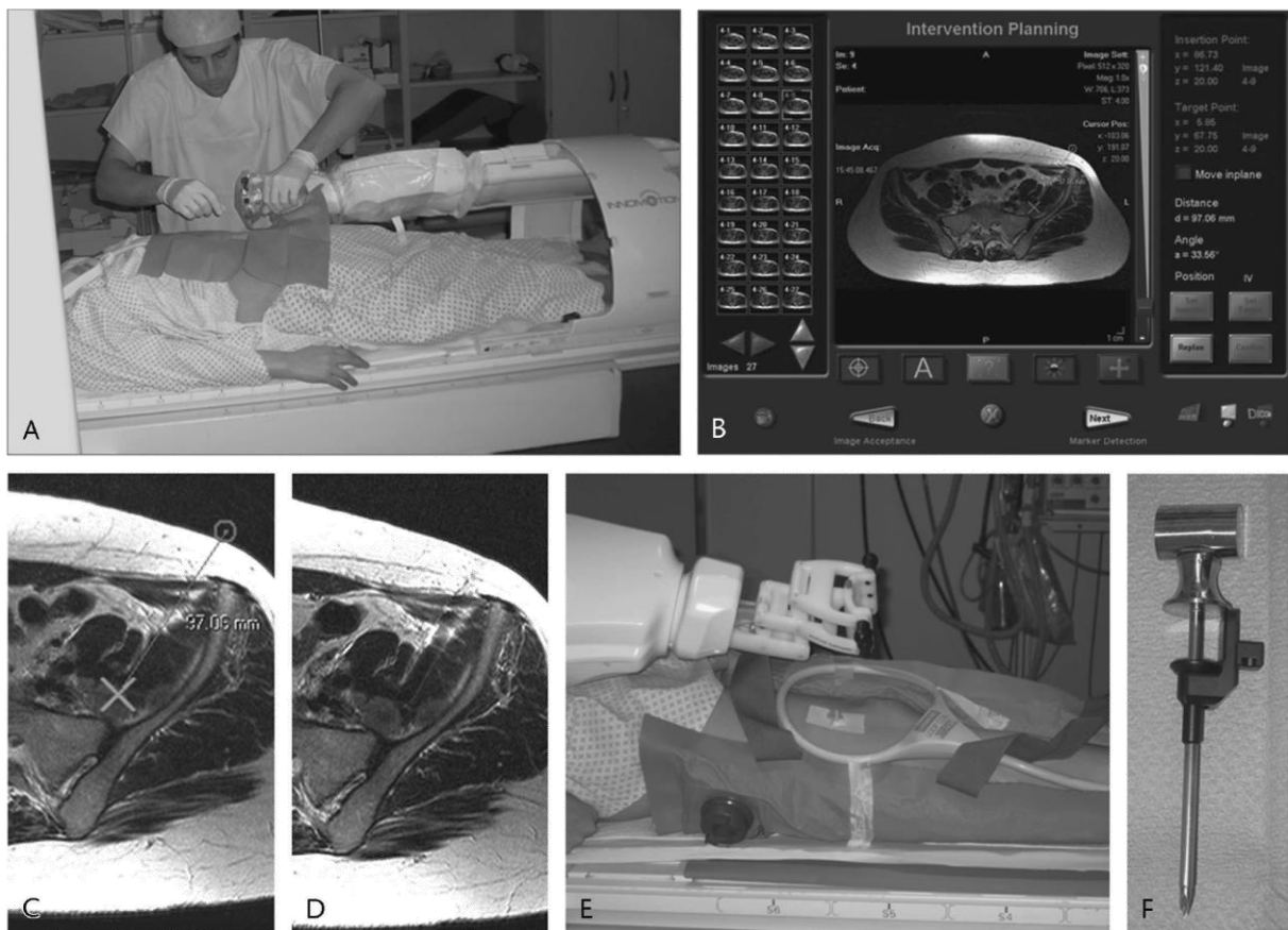
FIGURE 6. Magnetic resonance-compatible robotic manipulator for percutaneous procedures in a closed-bore cylindrical magnet. A, Clinical example I: soft-tissue biopsy of iliac lymph node in a 38-year-old woman with known cervical cancer. Clinical setup with robotic C-arm locked on MR table and application module (AMO) already moved into initial position. A sterile cover is placed over AMO and robotic arm. B, Screenshot of user interface on standalone control PC divided into areas for MR image selection, graphical trajectory planning, and numerical coordinate information and with general control buttons. Planned needle position and direction are then accurately realized by pneumatic actuators and optical sensors. C, Detail of B indicating planned needle path with entry point (circle), target point (X), and insertion depth. After MRI verification of the direction, needle is inserted manually outside the bore. D, Control MR image showing coaxial needle in final position for biopsy. E, Clinical example II: bone biopsy in the distal right femur of a 37-year-old woman with persistent pain when walking. Suspicious lesion was detected in bone scintigraphy but could neither be seen with conventional x-ray nor with CT. 22 Detail of clinical setup on MR table with right leg immobilized by vacuum mattress. A 19-cm-wide loop coil is used for MR signal reception. D, Bone biopsy set (Invivo) used for penetration of the cortical bone. Stylet and trocar are inserted through a guiding sleeve that attaches to the AMO of the robotic arm.
