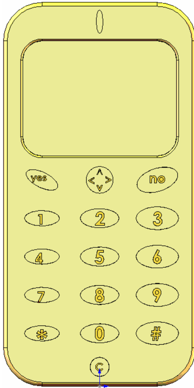
Figure 5.3 Asymmetric geometry (left buttons with smaller areas) yet symmetric color
