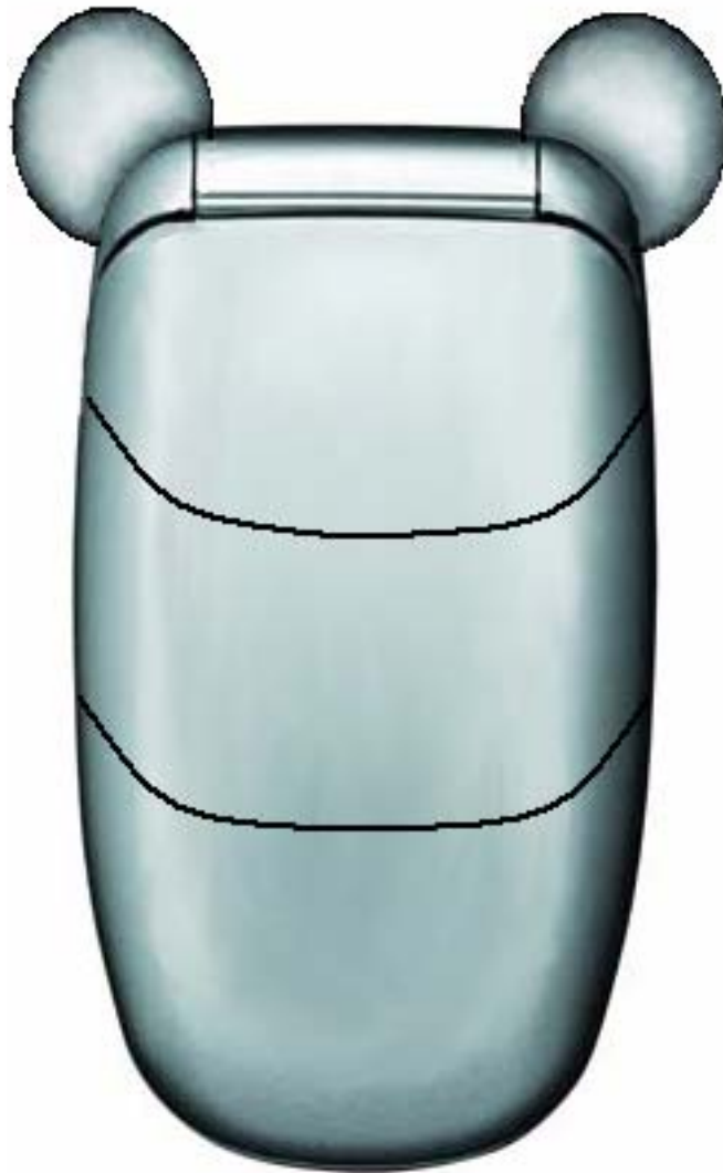
Figure 5.9 Cell phone picture with smile pattern and balance antenna
