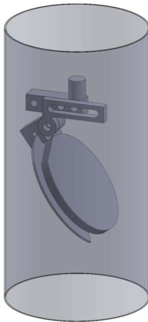
Figure 6.3 Illustration of the sample holder employed for mounting the Na 2 IrO 3 film stack within the 49 mm cryostat bore. The stack is glued onto a c-shaped piece of 0.5 mm-thick aluminum that can be fixed and tilted at an arbitrary angle. [Drawing by Pavlo Portnichenko, TU Dresden]
