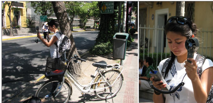
Figure 5.3: Manual measurements of air temperature and wind speed and direction using thermo-anemometer.
