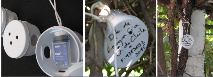
Figure 5.2: HOBO® installed within specifically designed weather-shelter.
