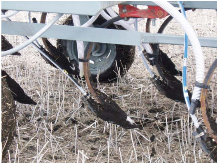
Figure 2. Modified drill for AA application at 10.5 cm (12 inches) spacing.
