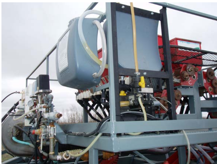
Figure 3. Attachment to allow direct injection of N-Serve into the AA stream.
