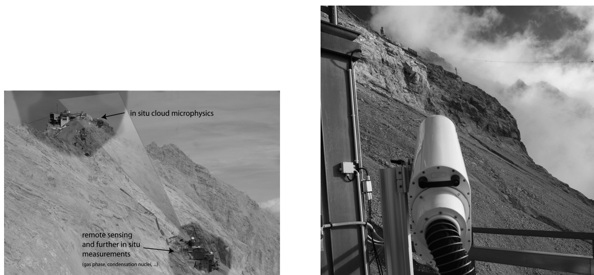
Fig.1: (left) Distribution of instruments between the Zugspitze summit and the environmental research station Schneefernerhaus. (right) : LIDAR observing clouds at the summit.
