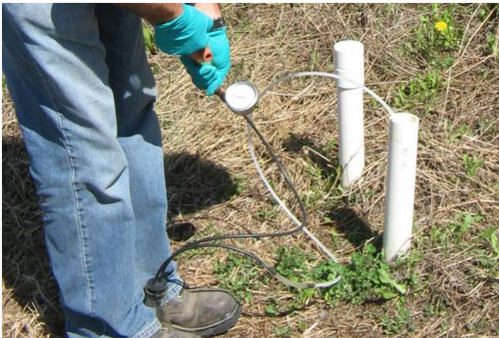
Figure 3.4: Water sample extraction from monitoring wells.
