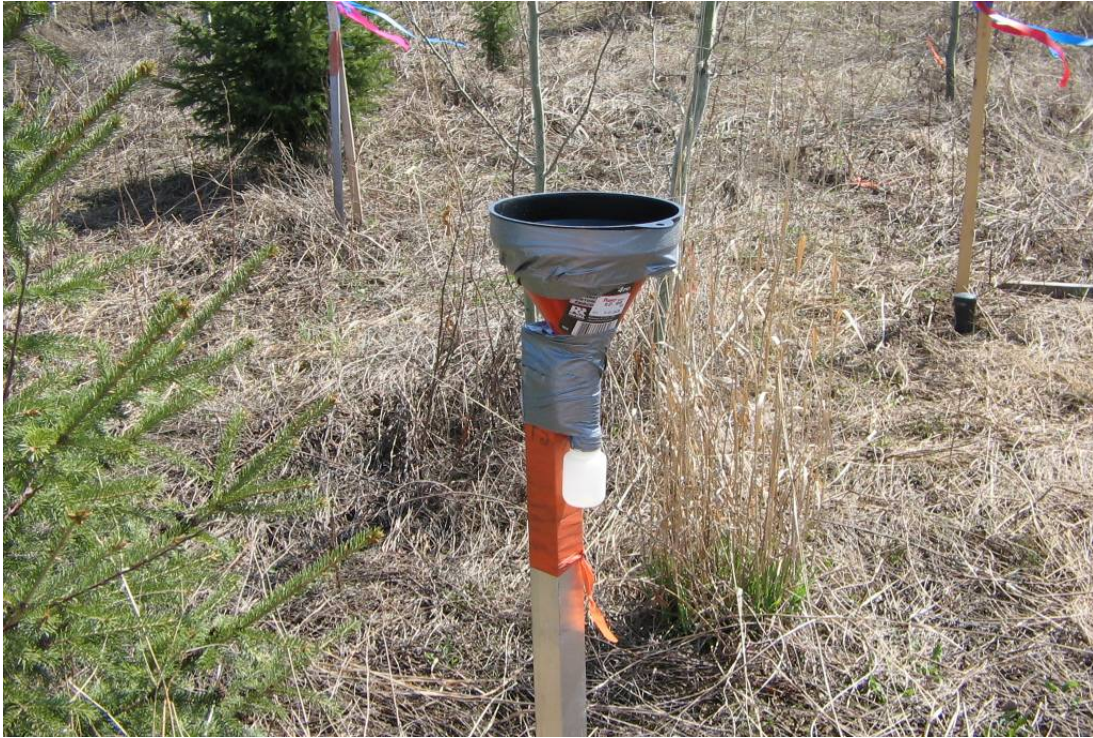
Figure 3.5: Precipitation sampling device.
