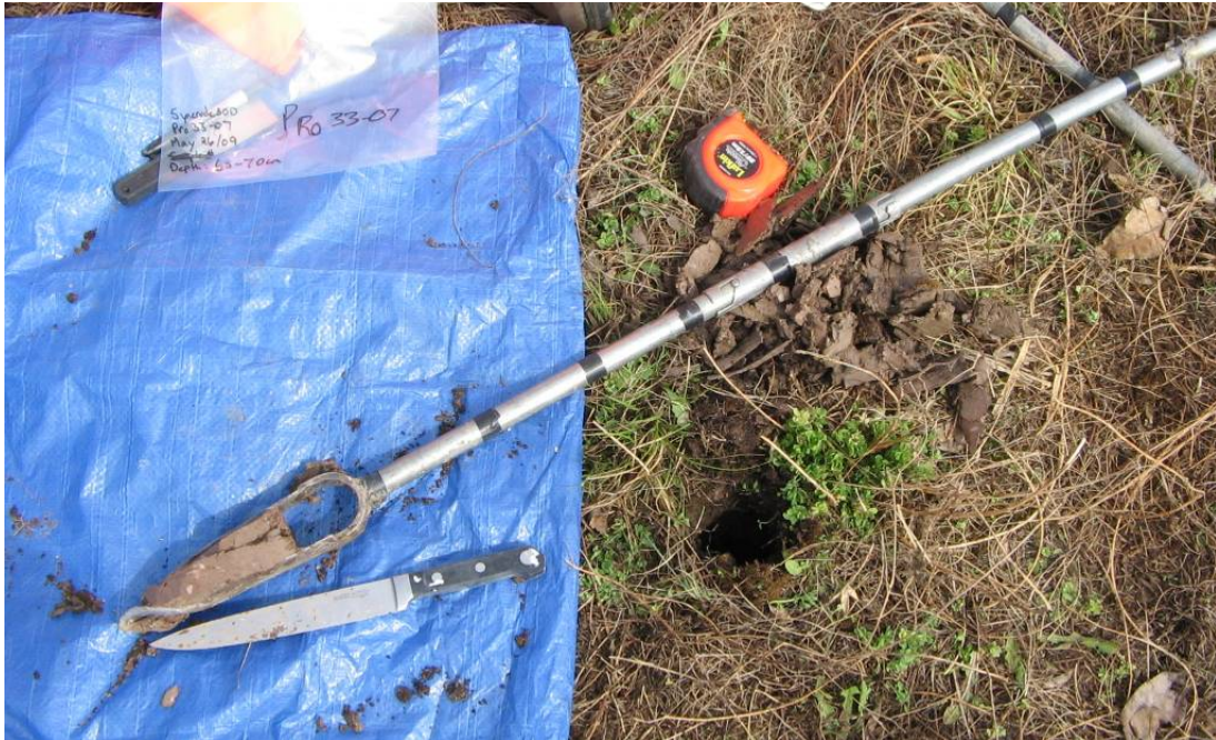
Figure 3.7: Dutch auger used for soil sample collection.
