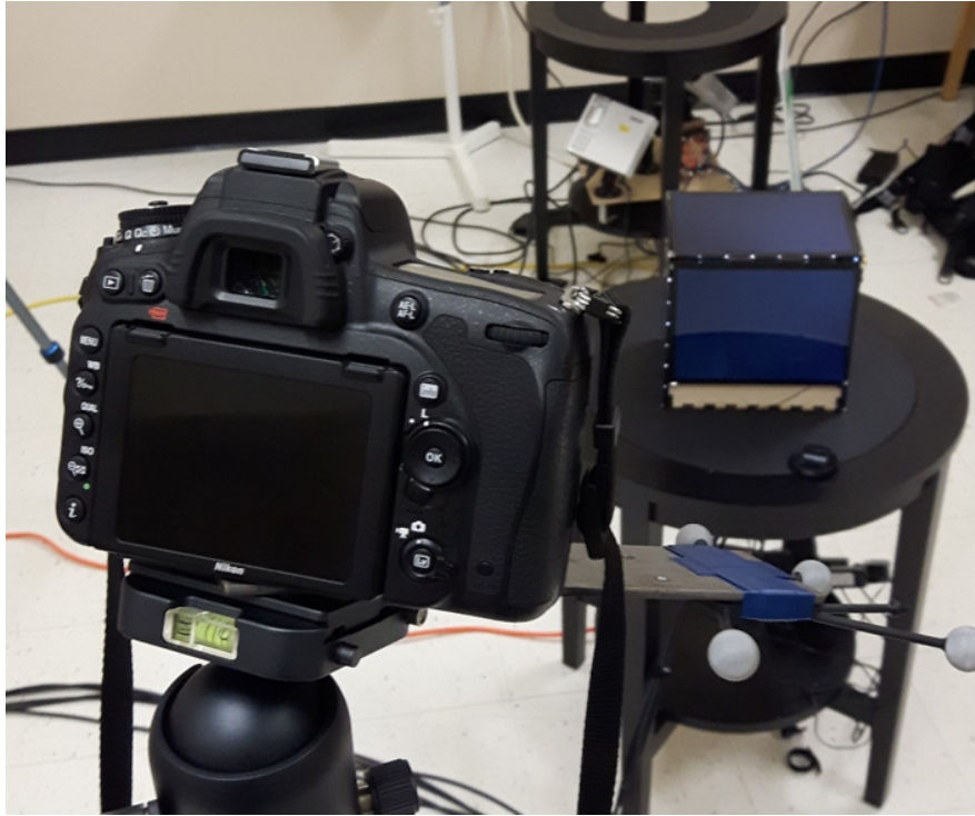
Figure 5.6: Tracked camera, used for calibration
