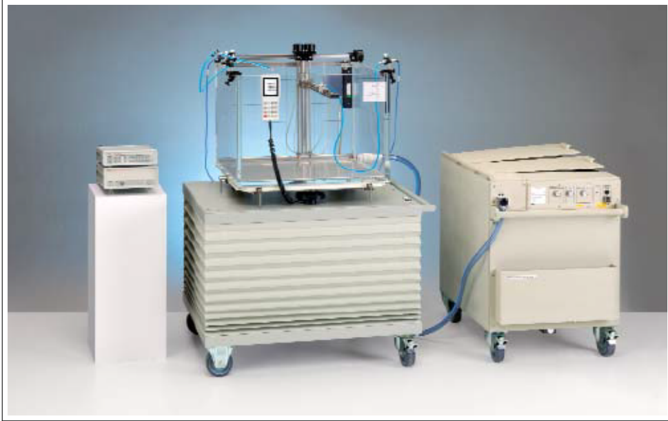
Figure 3.2: Large size motorized 3D water phantom system for dose distribution measurement of radiation therapy beams [15]
