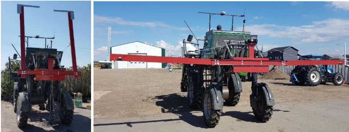
Figure E-1: mechanical boom in a) transportation position and b) data collection position
