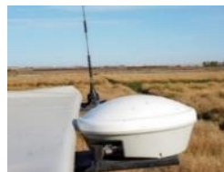
Figure 2-54: Utilized GPS antenna on the farm vehicle
