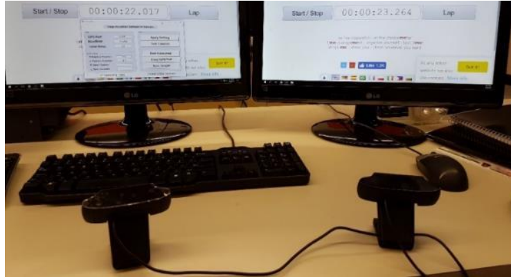
Figure 2-34: Assessing response time of the utilized webcams
