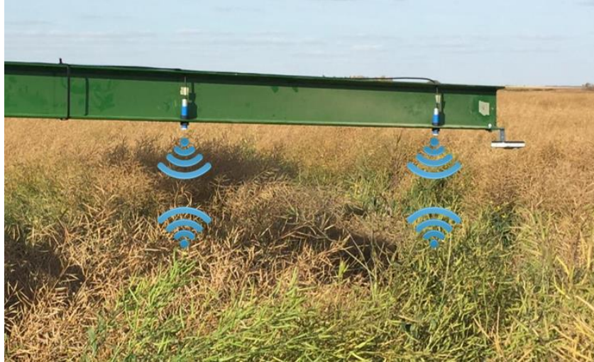
Figure 2-5: Using ultrasonic signal to measure height of a plant
