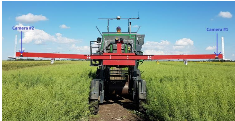
Figure 2-36: The location of utilized cameras on the boom
