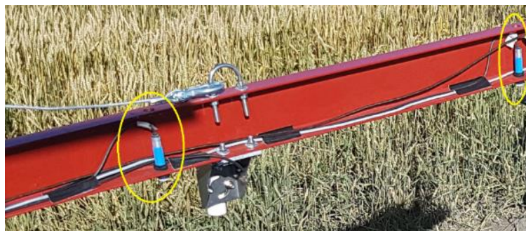
Figure 2-21: Closer view at utilized ultrasonic sensors on the boom
