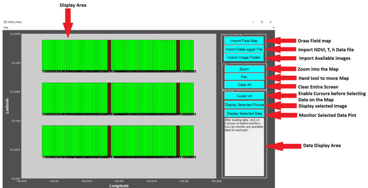
Figure 3-13: User interface for developed data visualization program
