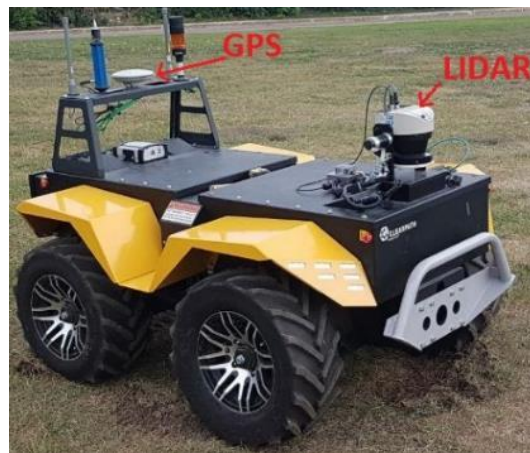
Figure 1-6: A typical autonomously navigated robot for plant phenotyping
