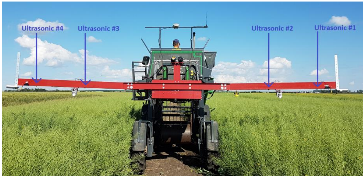
Figure 2-20: Utilized ultrasonic sensors on the proposed HTPP
