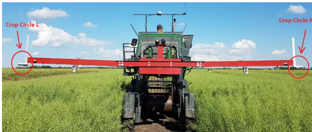
Figure 2-46: Location of NDVI sensors on the back boom
