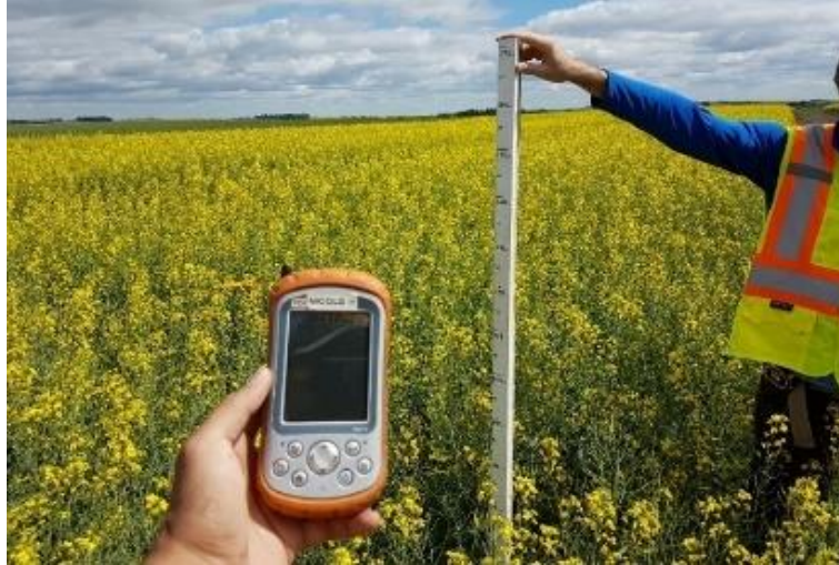
Figure 4-33: Manual height measurement for verifying ultrasonic height measurements
