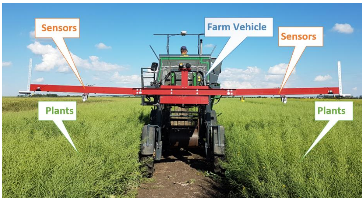
Figure 1-4: Using a farm vehicle and a boom for plant phenotyping
