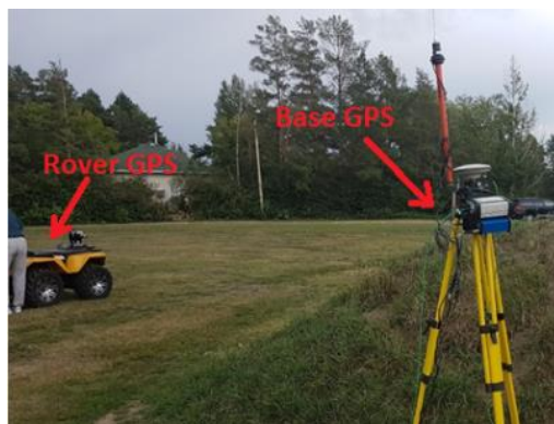
Figure 2-52: An RTK GPS system
