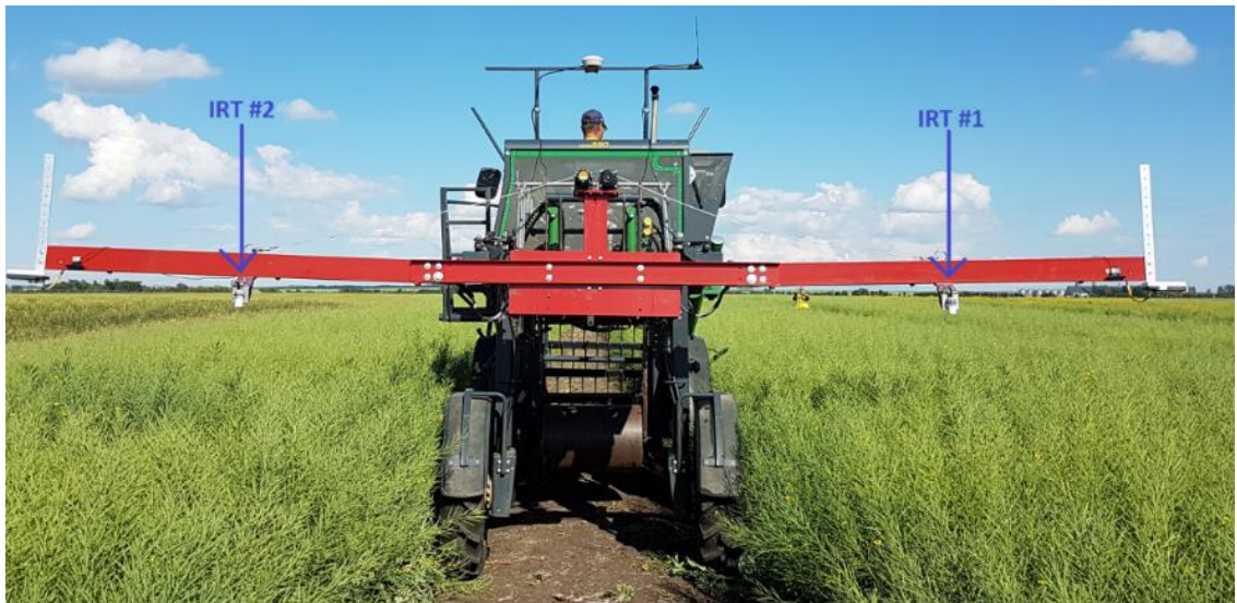
Figure 2-29: Utilized IR thermometers on the proposed HTPP
