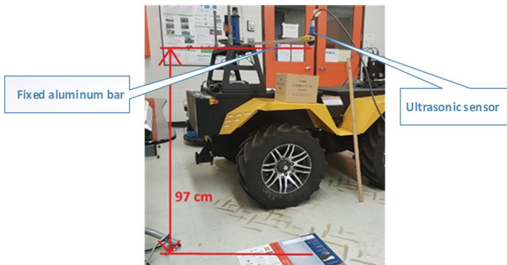
Figure 2-9: Sensor attachment for calibration
