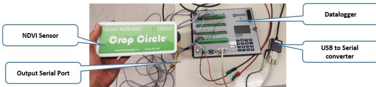
Figure 2-44: Performance assessment of the utilized sensor in laboratory configuration
