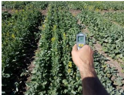
Figure 2-23: A portable non-contact temperature measurement device
