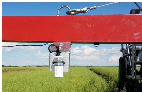
Figure 2-30: Closer view at utilized thermometer on the boom
