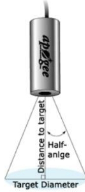
Figure 2-25: Field of view of the utilized thermometer
