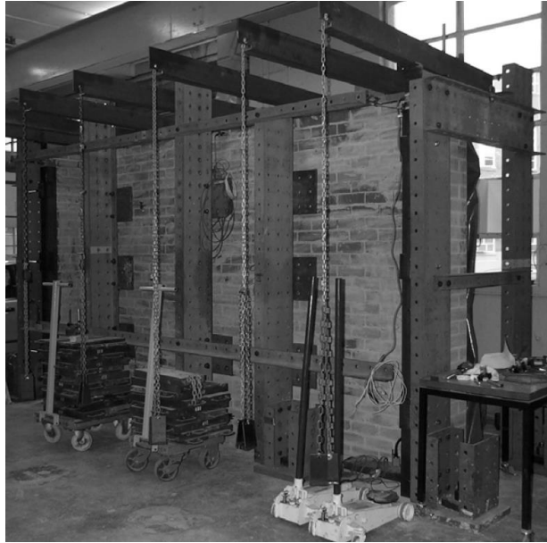
Figure 2.9: Masonry wall test set-up (Griffith & Vaculik. 2005).
