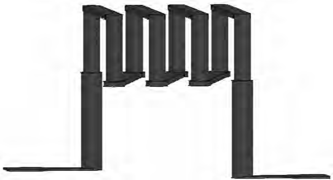
Figure 2.14: Suspended solenoid inductor with 150 \mu m air gap
