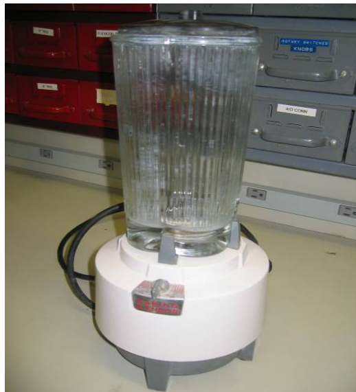
Figure 4.1. High Speed Blender used for mixing of cement paste
