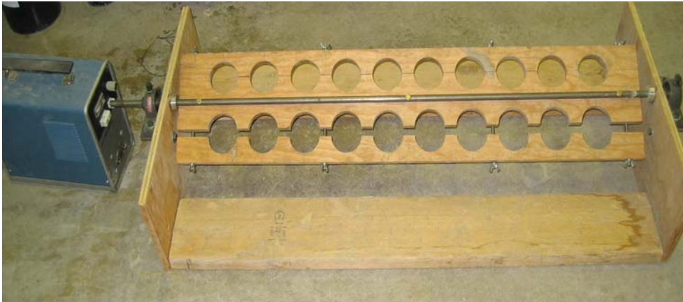
Figure 4.2: Rotating device used to prevent segregation
