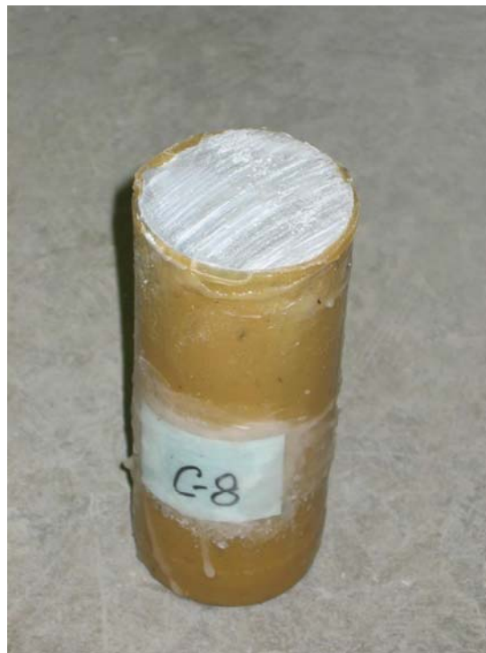
Figure 4.6: Sample cylinders coated with paraffin wax.
