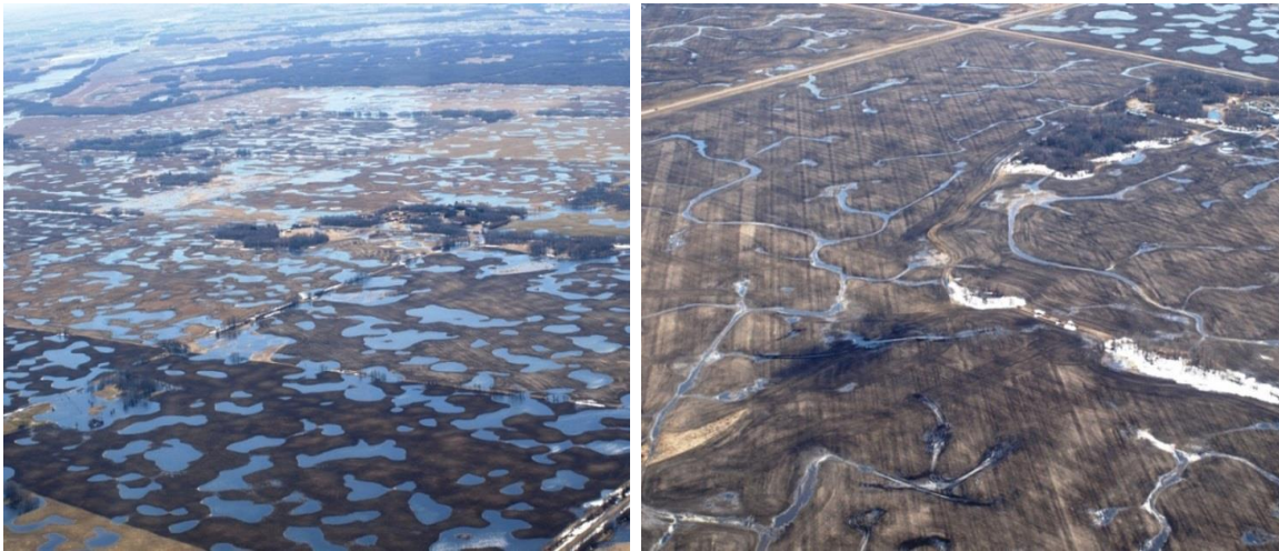
Figure B.1: Aerial photographs from Smith Creek Research Basin on April 28th, 2011. [Right] An area of SCRB where no drainage has occurred and the surface runoff generated is stored in the depressions on the landscape. [Left] An area of SCRB where wetlands have been drained and the surface runoff is no longer stored on the landscape, but follows the drainage channels to ditches or streams. Photo Credit: Ducks Unlimited Canada.
