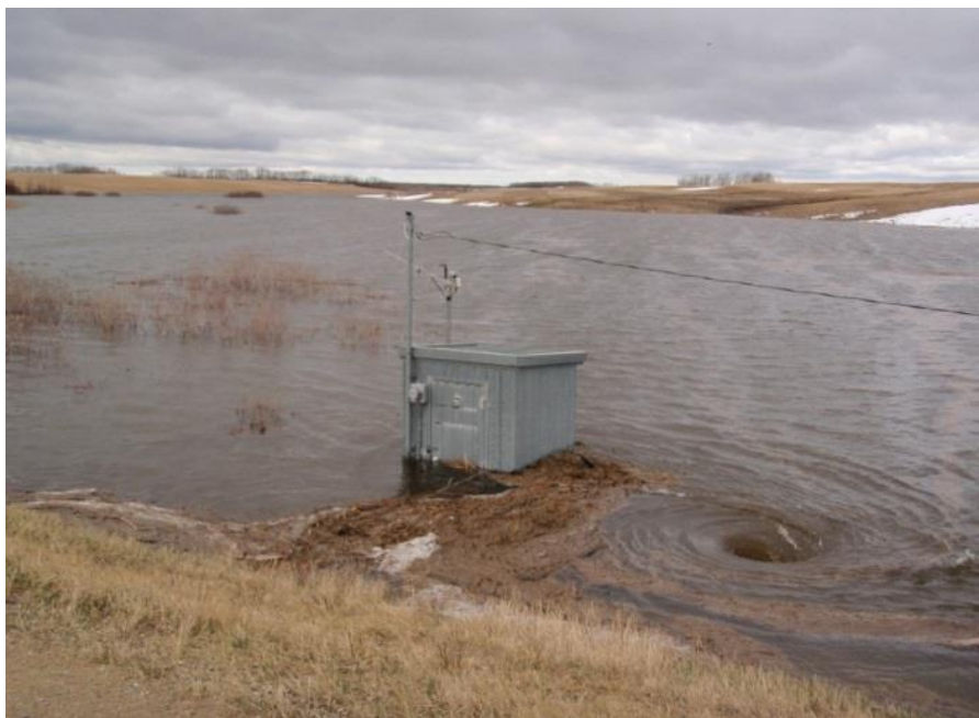
Figure B.4: Photograph looking upstream of the outlet of SCRB. Taken May 4, 2011 during a rain-on-snow flood event (1 day before peak). Photo credit: Nicole Seitz.
