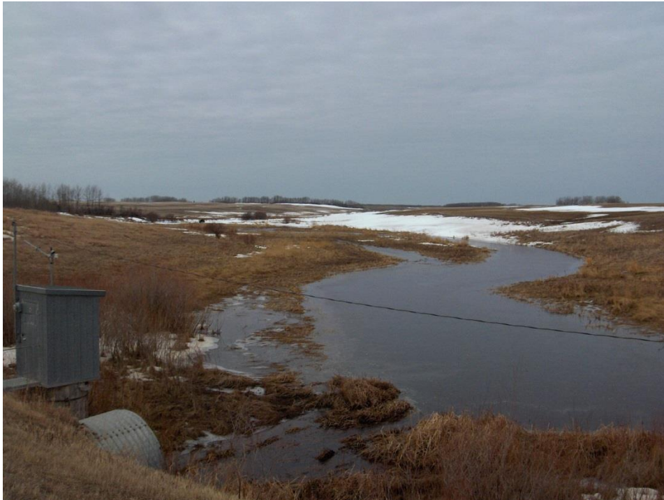
Figure B.8: Photograph taken on April 13, 2008 (2 days prior to peak flow). Shown as a reference photograph for the outlet of the SCRБ under average flow conditions during spring freshet. The culvert and height of the hydrometric station can be seen in this photo. Photo credit: Logan Fang.
