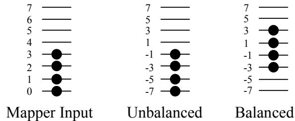
Figure 3.5: Mapper Input and Mapped Levels for QAM-16 ( N/2=2 , N_{max}/2=3 )
