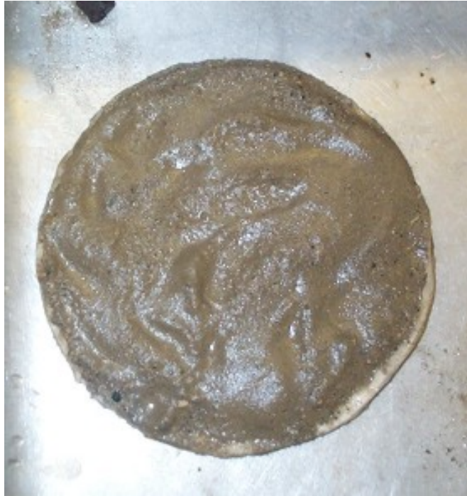
Figure 5.8 Geotextile clogged with fines originating from sieved, but not washed, crushed concrete.
