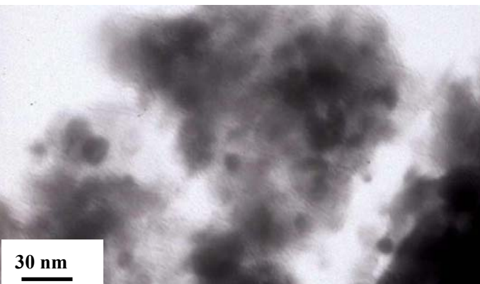
Fig. 4.14 TEM images of different Ni-Co content catalysts after 250 h TOS
