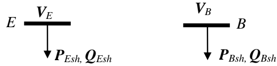
Figure 2.6: VSC HVDC link equivalent circuit for load flow studies and steady-state analysis.
