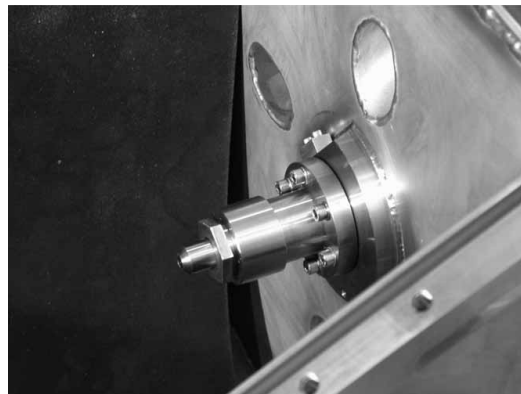
Fig. 6. The exit nozzle mounted at the beam entrance in the chamber.
