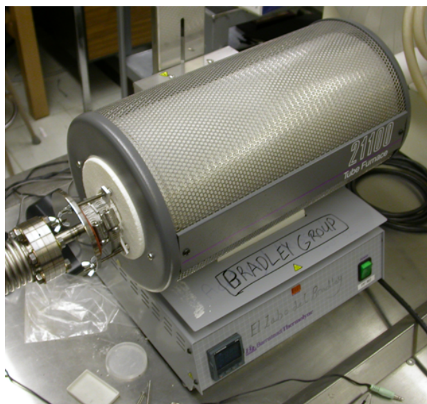
Figure 4.9: The Thermolyne 21100 tube furnace used in the present research. The metal hose attached to the left side of the tube connects to the front of the vacuum chamber to allow the tube to be evacuated during the annealing process.
