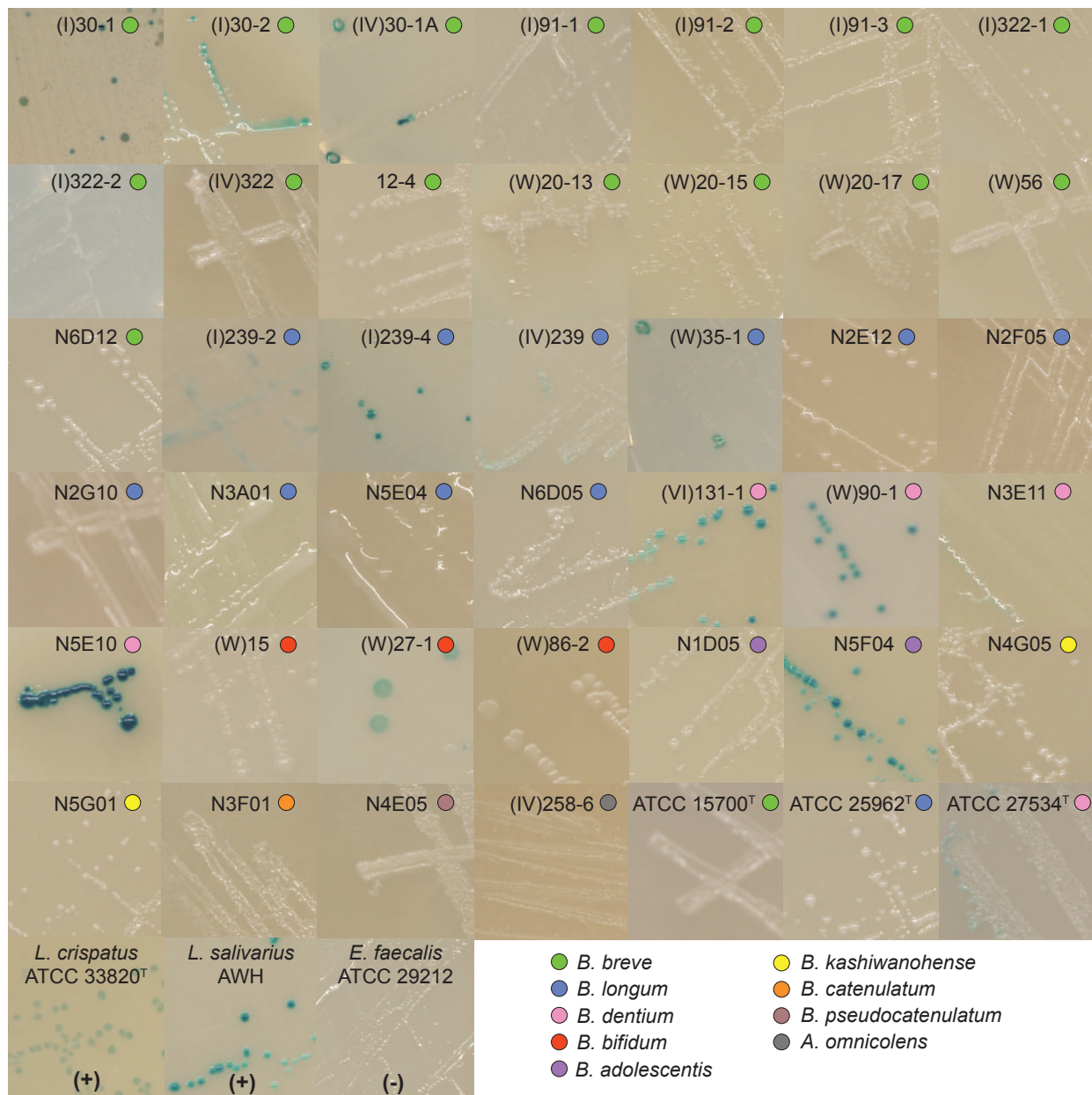
Figure 4.4. Hydrogen peroxide production indicated by blue colour on TMB medium.
