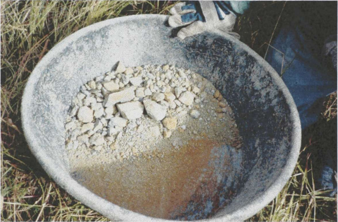
Figure 4.3 Cuttings from a Becker Hammer drill rig.
