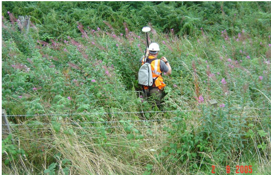
Figure 3.4: dGPS roamer unit in use at Adavoyle bog site, cross sections of embankments being taken.
