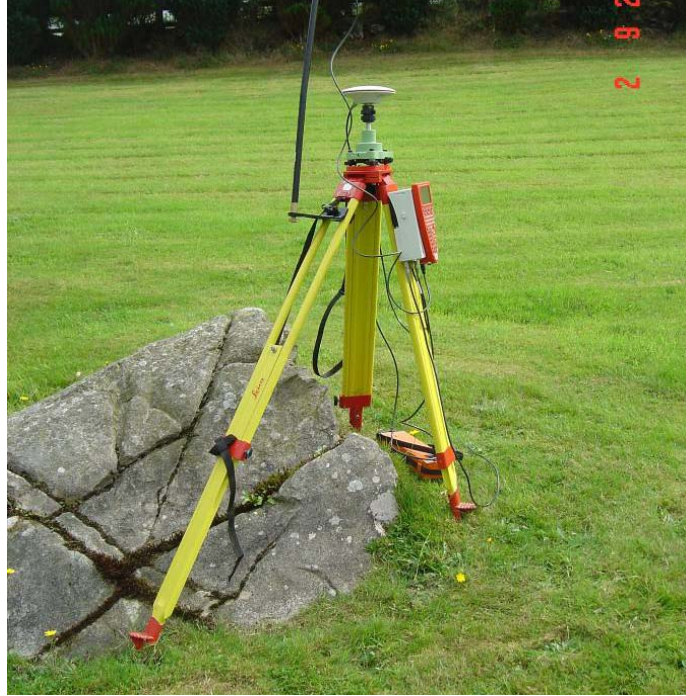
Figure 3.3: dGPS base station set up in private yard adjacent to Adavoyle bog site.
