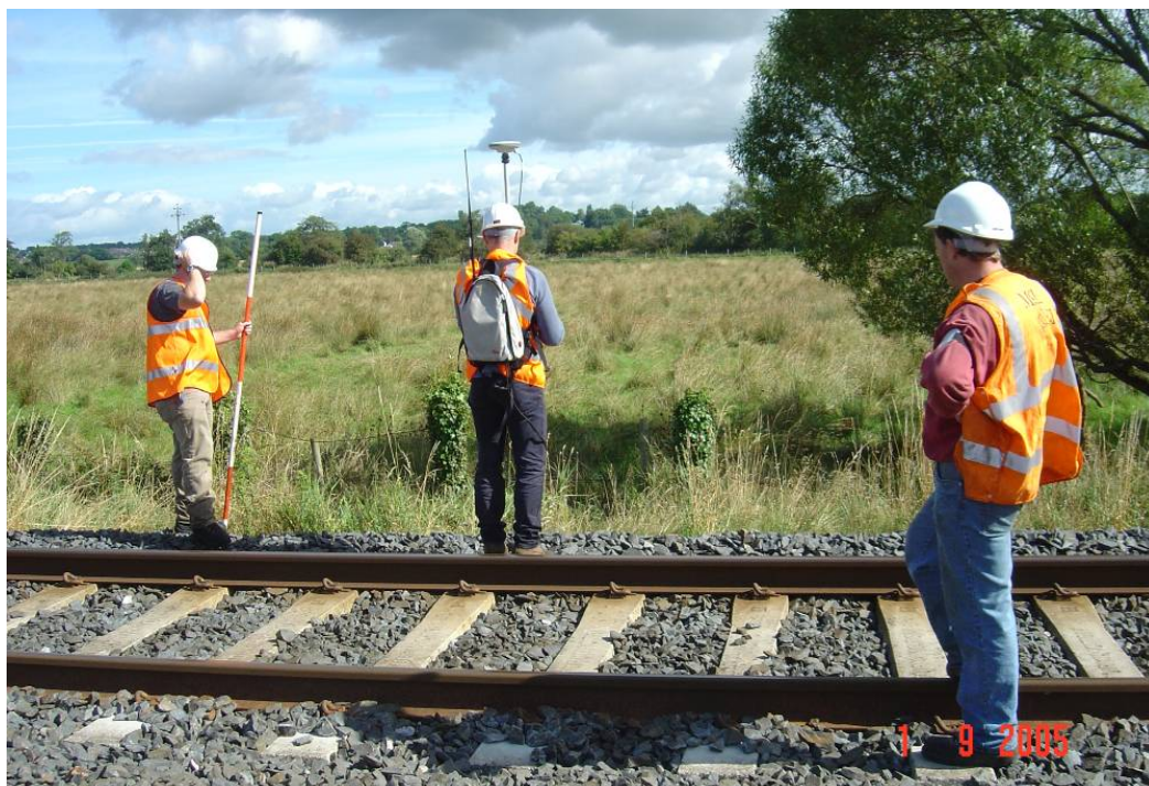
Figure 3.2: dGPS roamer unit in use at Brackagh bog site, cross sections of embankments being taken.
