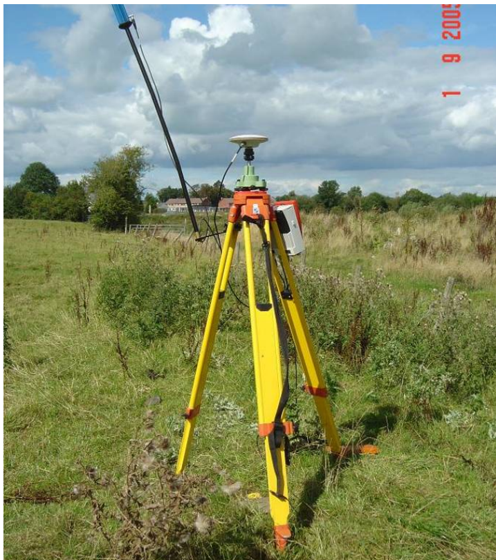
Figure 3.1: dGPS base station set up in field adjacent to Brackagh bog site.
