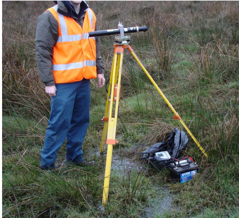
Figure 3.5: Laser set-up on tripod in field at Brackagh bog site
