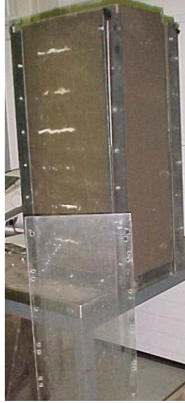
Figure 3.8 Soil column inside the Plexiglas ® container after removing one side of the container.
