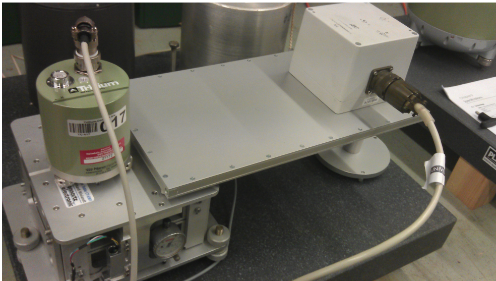
Figure 3.7: Laboratory test of the Eentec R2 rotational motion sensor. Comparison of the rotational motion sensor R2 (right) with a Nanometric Trillium seismometer (left). The seismometer is placed on a Lennartz step table, the R2 sensor is located on a bridge with arm length of 396.5 mm. In this test the generator constant and the phase shift for the different axes of the R2 sensor in multiple frequency bands are determined.
