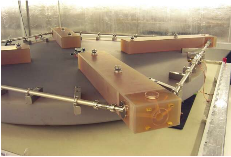
Figure 3.2: Ringlaser gyroscope in Wettzell. The sensor is installed at the geodetic observatory and measures changes in the rotation rate due to changes in the Earth's rotation or due to seismic waves (Wettzell, 2015). Clearly visible are the four sides of the cavity, hosting the counter propagating laser beams, with a length of 4 m each. This results in a sensor surface of 16 m 2 and a perimeter of 16 m.
