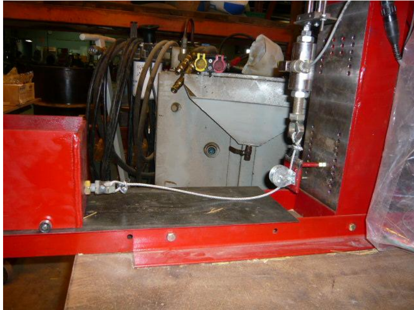
Figure B.3 Photograph of the dynamic coefficient of friction tool installed on the material properties test stand.
