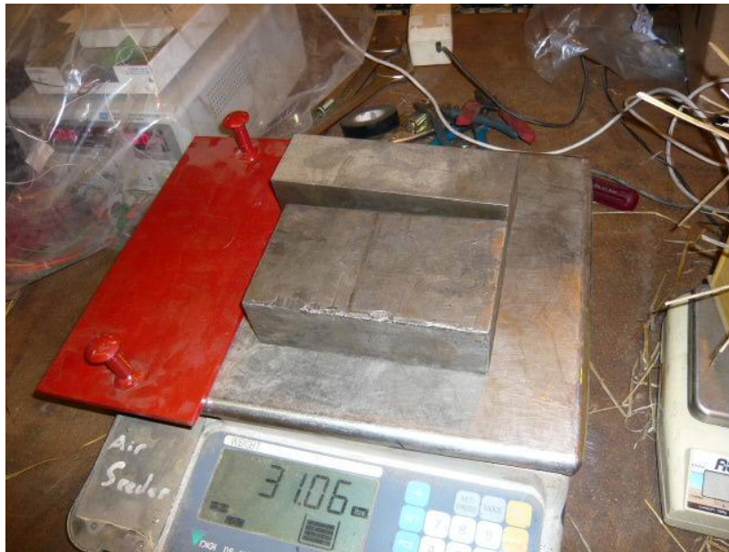
Figure B.5 Photograph of the compression plate and weights used to load the material to determine the dynamic coefficient of friction.
