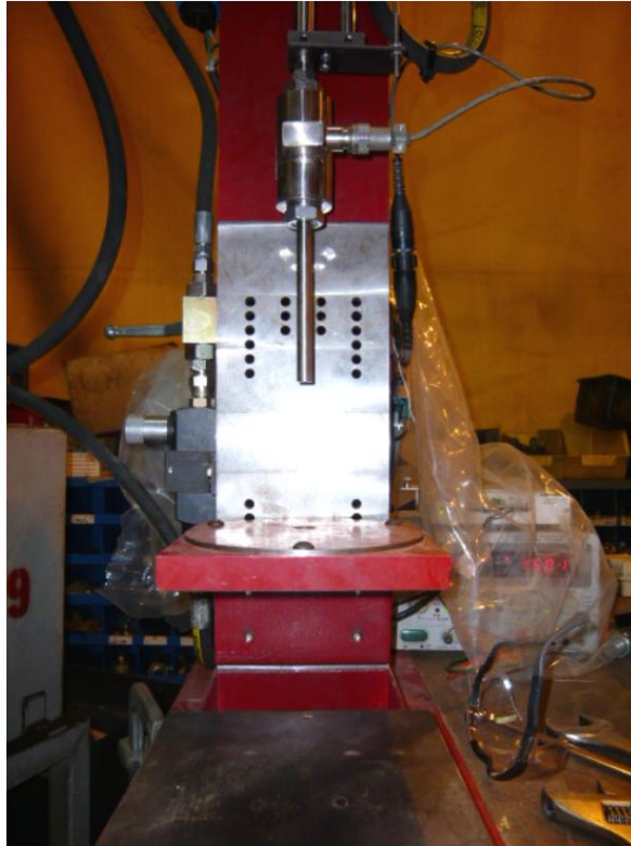
Figure B.9 Photograph of the plunger and die used to determine the maximum shear strength installed on the material properties test stand.
