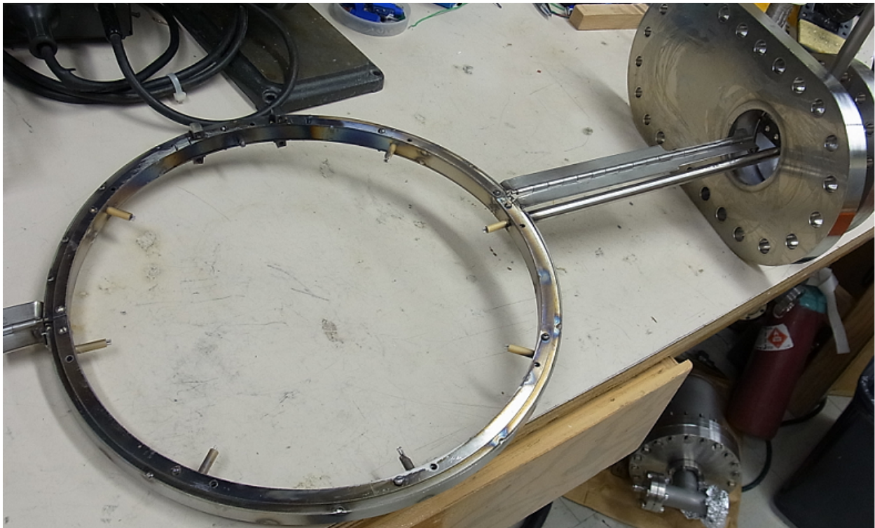
Figure 5.7: Used probes ring for GAM identification experiments in STOR-M.
