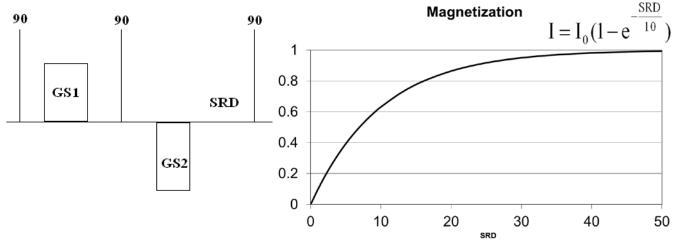
Figure 2.1 The spoiler recovery sequence and a plot of the magnetization after a variable delay SRD.
