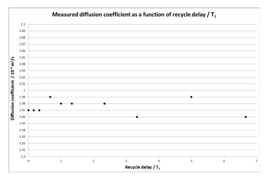
Figure 4.5 Varying the recycle delay on a doped water sample ( $T_1 \sim 300 \text{ ms}$ ) using the spoiler recovery 13-interval PFGSTE.
