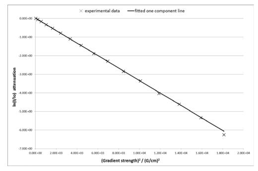
Figure 4.4 Application of the combined spoiler recovery 13-interval PFGSTE on pure water at 11.7 Tesla.
