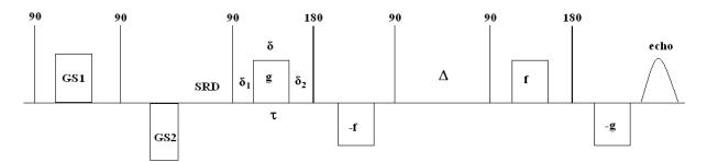
Figure 4.3 The combined spoiler recovery 13-interval PFGSTE sequence
