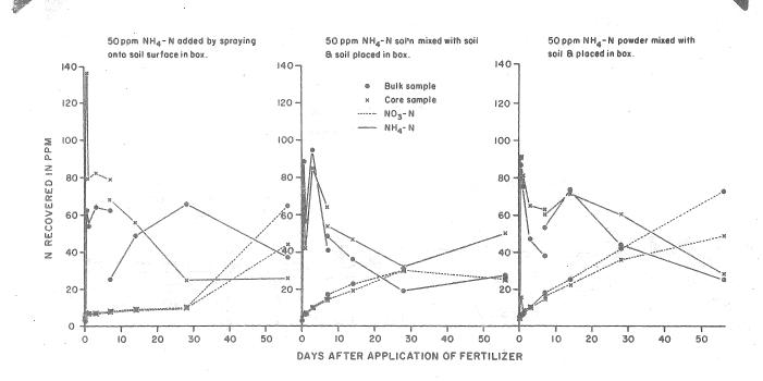
Fig. 3. Effect of methods of application and sampling on recovery of fertilizer N - NH<sub>4</sub>-N applied.
