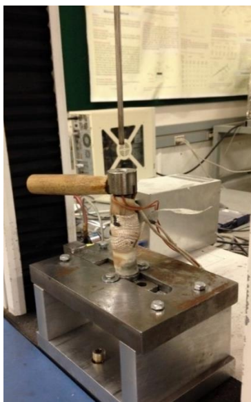
Figure 4.2: Single pelleting unit mounted on an Instron Model No.3366 tester for pelleting of samples.
