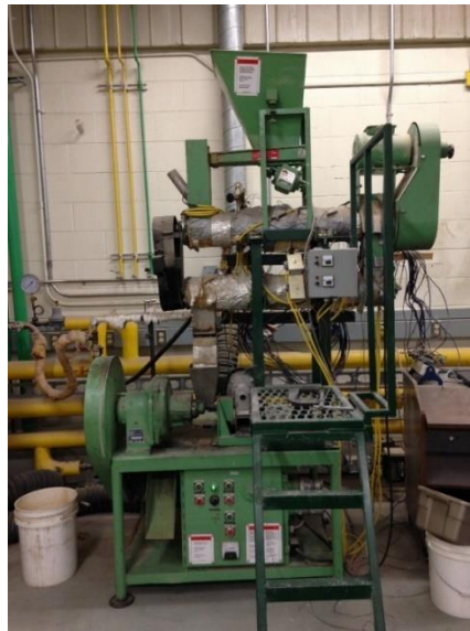
Figure 4.4: CPM-CL5 pilot-scale pelleting unit used for pelletizing samples.
