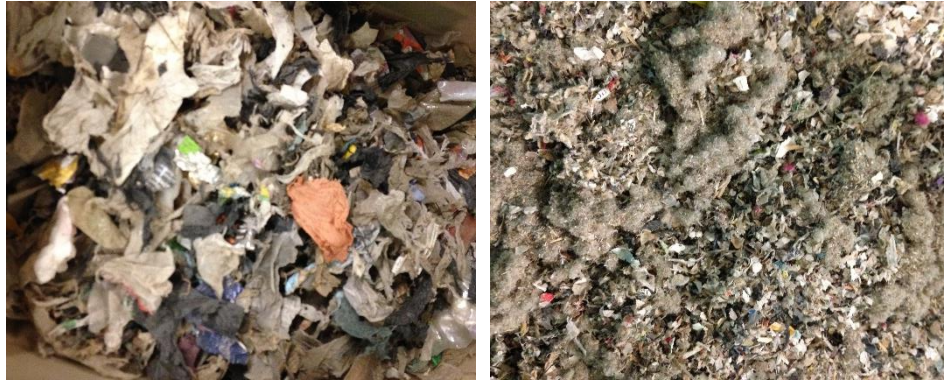
Figure 4.1: Example of RDF-fluff before (left) and after (right) particle size reduction using a knife mill fitted with a 6.35 mm screen.
