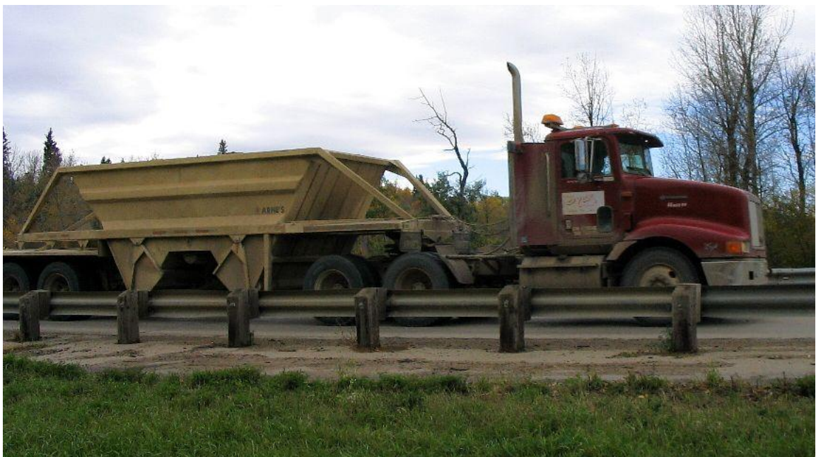
Figure 3.20 Test truck used for static load test.
