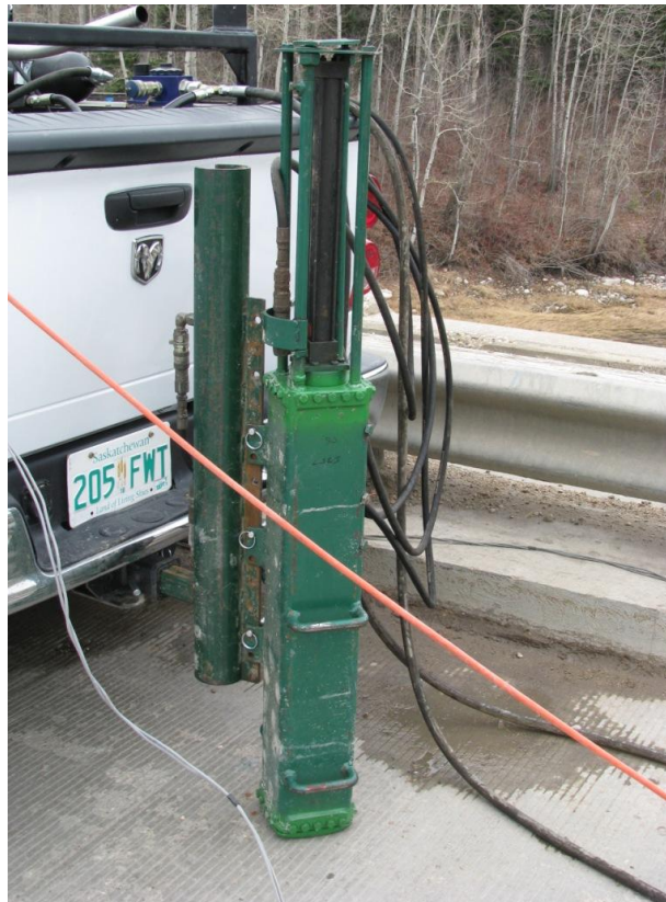
Figure 3.16 Spring actuated impact hammer mounted on the back of a truck.
