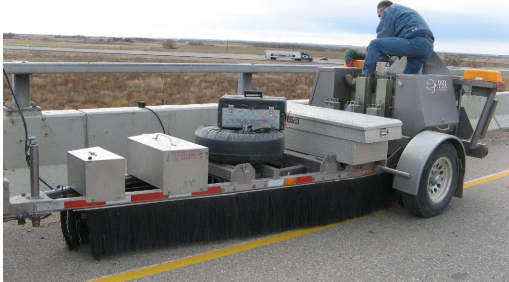
Figure 3.22 Heavy Weight Deflectometer (HWD).
