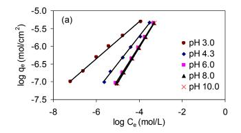
Figure 1: pH effect on 2,4-dinitrophenol adsorption isotherms of NTR 7450 membrane
