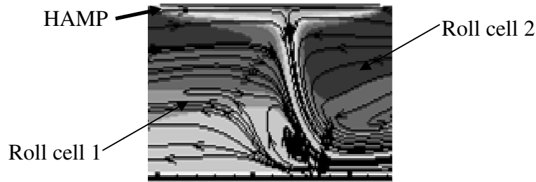
FIGURE 5.9. CFD simulation of streamlines and temperature gradient for unstable laminar airflow through the test section at t = 40 s, where the light color background is the coolest temperature and the darker color is the warmest temperature ( Re = 65 , Ra^+ = 37 \times 10^5 ).
