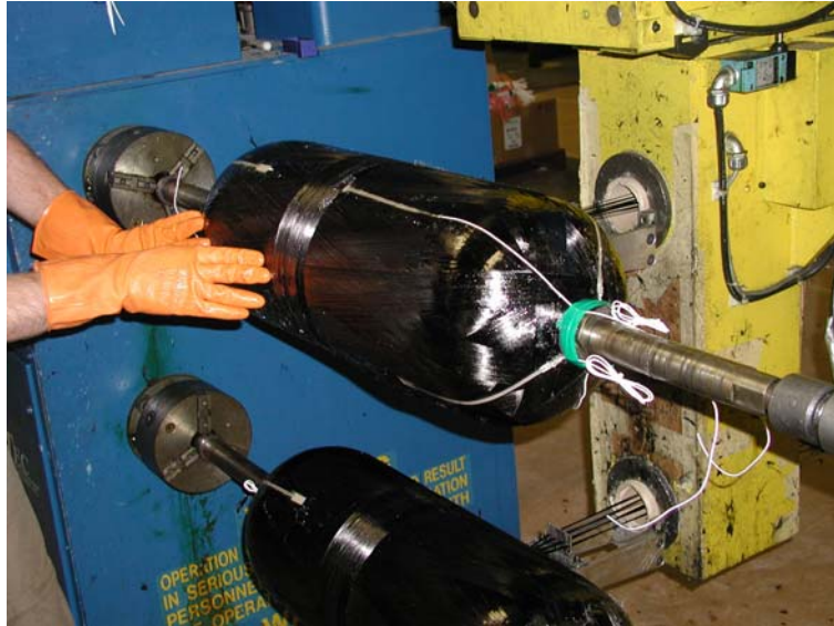
Figure 3.16: Embedded Sensor Final Design Manufacture
