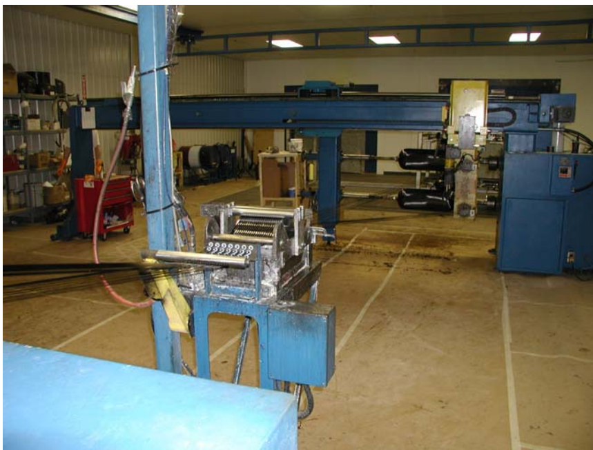
Figure C.2: Computerized Winding Machine
