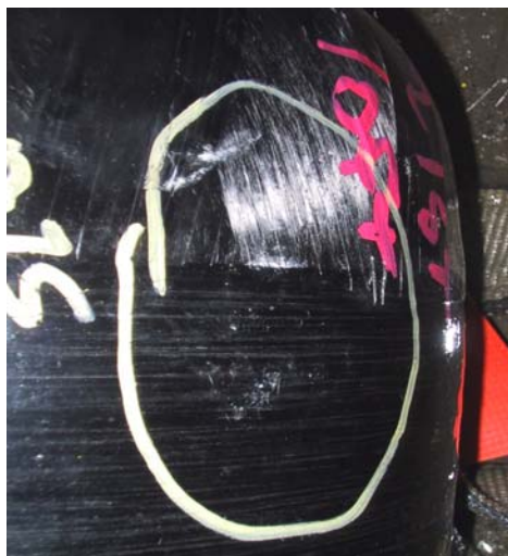
Figure 6.6: Tank Delamination Damage
