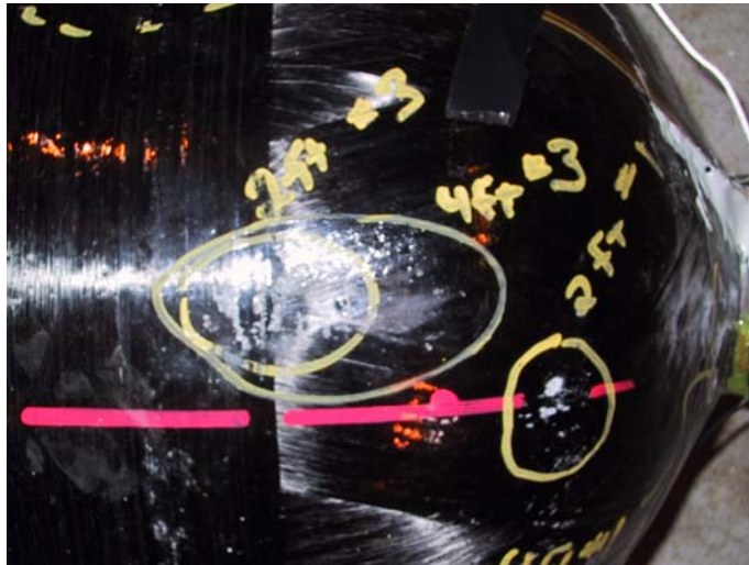
Figure 6.16: Delamination Damage from 1.8 m (6 ft) Drop
