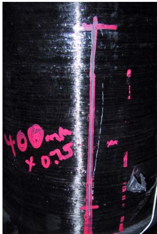
Figure 2.2: Typical Cut and Gouge Testing
