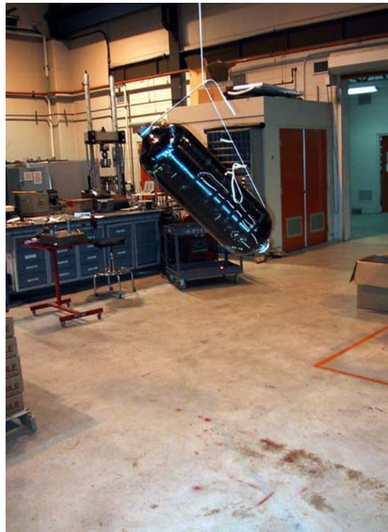
Figure 6.15: Drop Impact from 1.8 m (6 ft) onto Smooth Concrete
