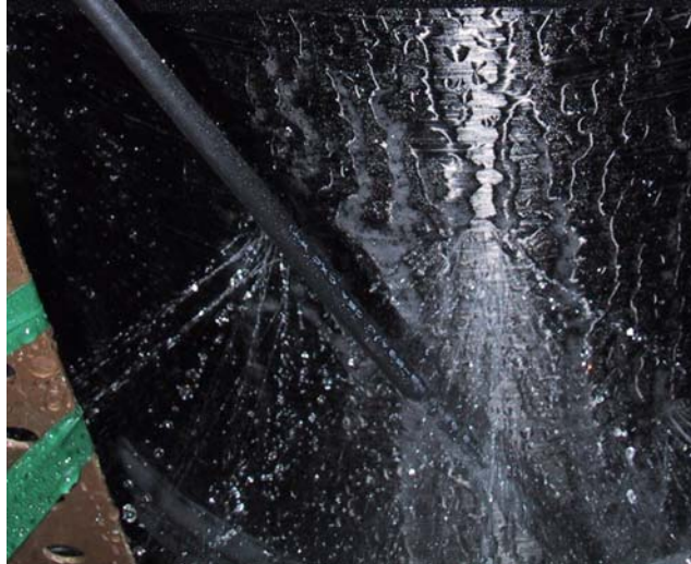
Figure 6.19: Fatigue Failure of Tank after 17,500 Pressure Cycles
