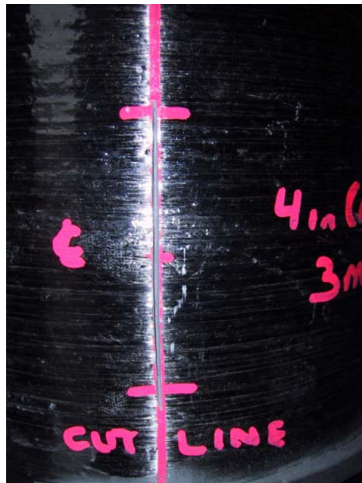
Figure 6.18: Cut #2 – 100mm (4 in.) Long by 4.5mm (0.18 in.) Deep
