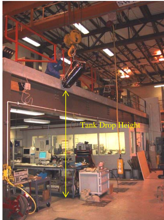
Figure 6.7: Tank Drop Height of 3.05m (10 ft)
