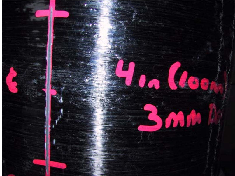
Figure 6.17: Cut #1 – 100 mm (4 in.) Long by 3 mm (0.11 in.) Deep
