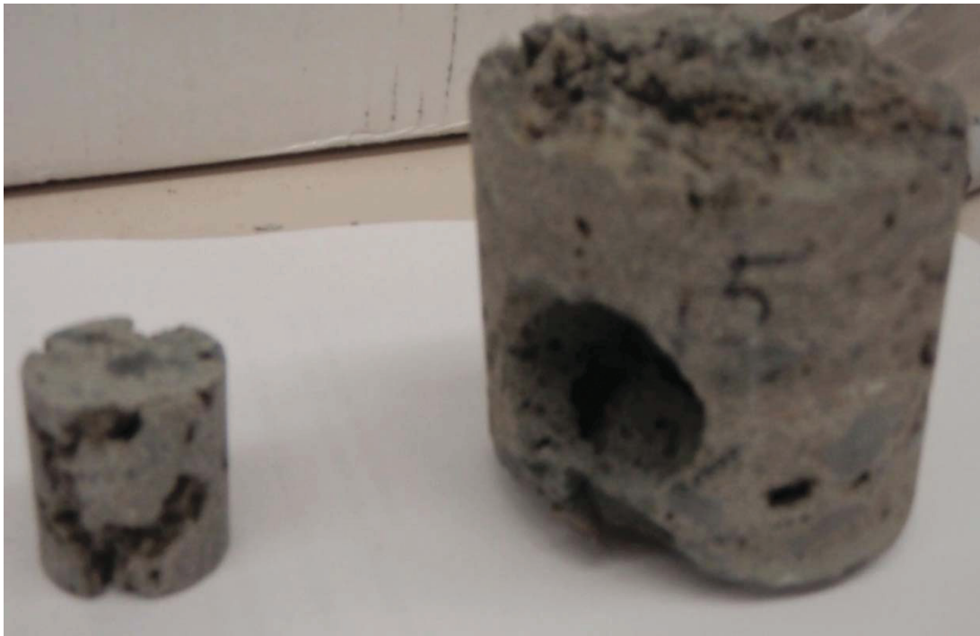
Figure 5.6 - Sample 5; sandstone with well-connected vugs (Scale: diameter of the plug on the left is 2.54 cm)
