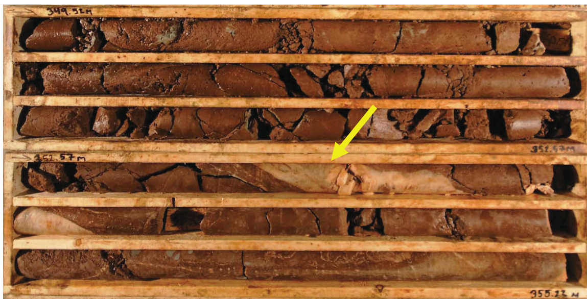
Figure 5.18 - PCS 0601 core from 349.52 - 355.22 m. The yellow arrow indicates the top of the gypsum-infilled zone (Photograph courtesy of PCS)
