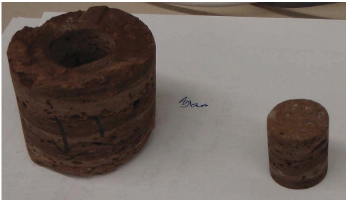
Figure 5.4 - Sample 1, cut perpendicular to bedding planes (Scale: diameter of plug is 2.54 cm)
