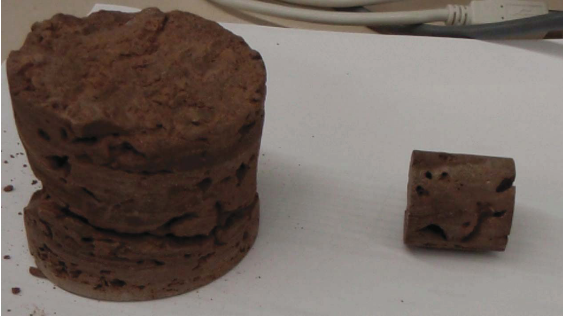
Figure 5.2 - Sample 1, cut parallel to bedding planes, prior to testing (Scale: diameter of the plug on the right is 2.54 cm)
