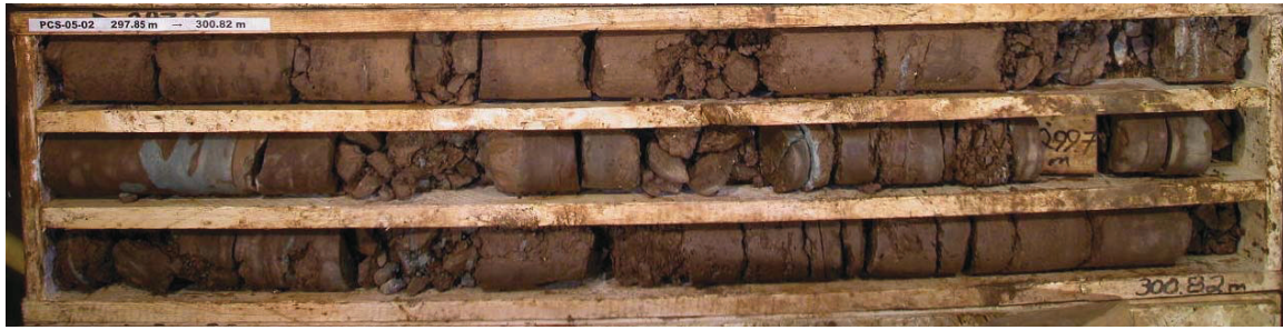
Figure 5.14 - PCS 0502 Core photo 297.85 to 300.82 m (RQD of 48%) (Photograph courtesy of PCS)
