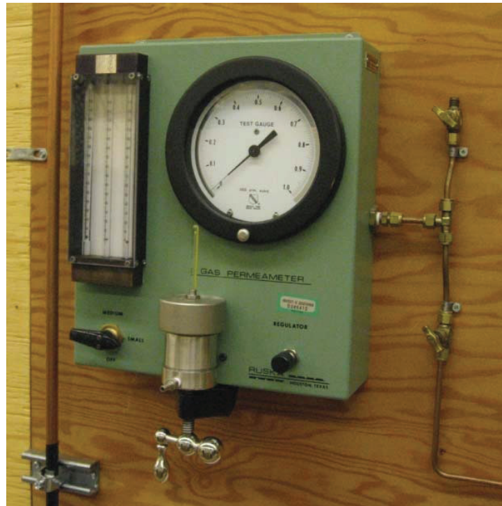
Figure 5.7 - Ruska gas permeameter
