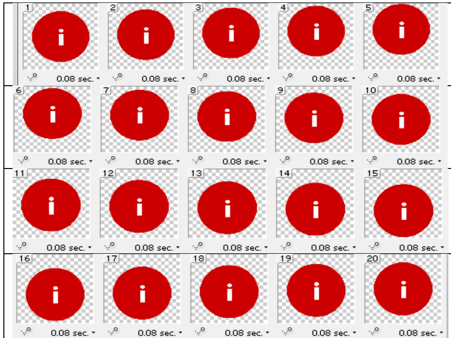
Figure 16: Frames of “Bounce” visual signal along with time allocated for each frame.
