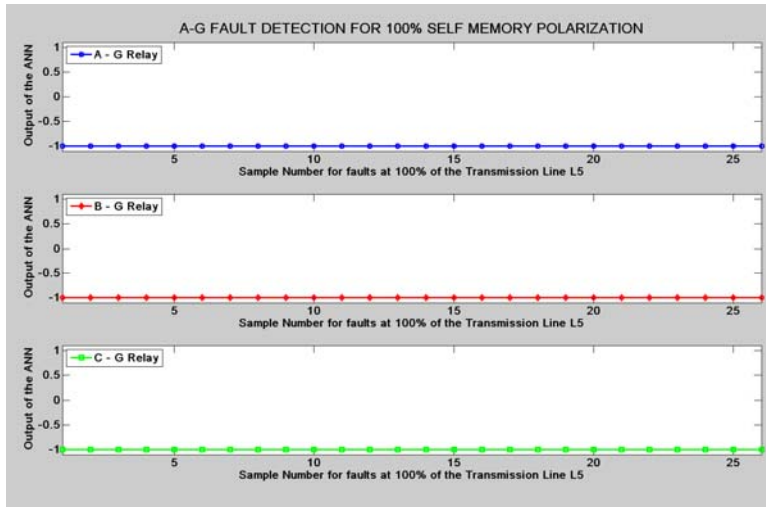
Figure G.152: Mho Relay – SLG Fault at 100% length of L_5 with 100% Self Memory Polarization
