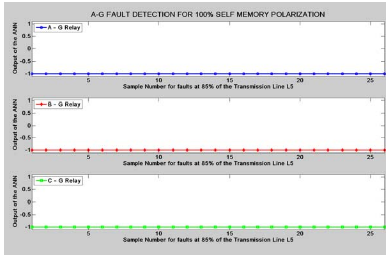
Figure G.149: Mho Relay – SLG Fault at 85% length of L_5 with 100% Self Memory Polarization
