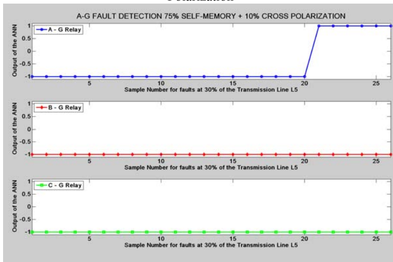
Figure G.183: Mho Relay – SLG Fault at 30% length of L_5 with 75% Self Memory + 10% Cross Polarization
