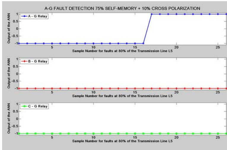
Figure G.194: Mho Relay – SLG Fault at 80% length of L_5 with 75% Self Memory + 10% Cross Polarization
