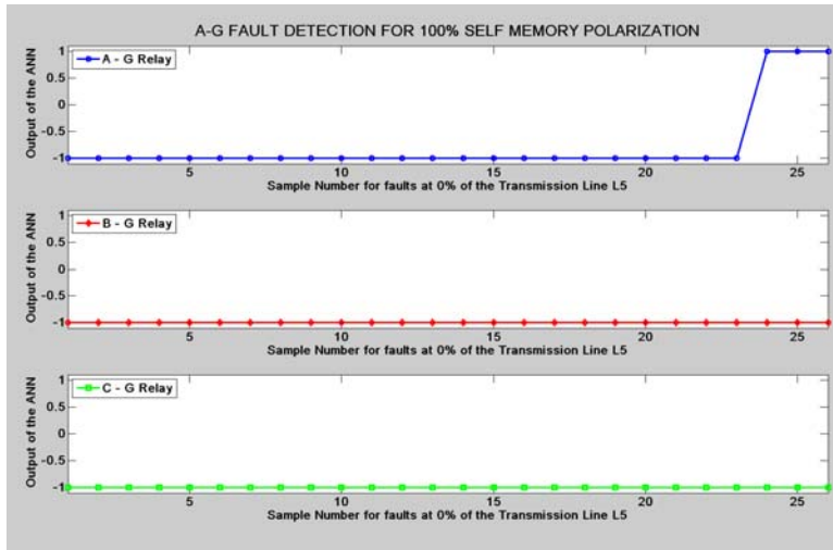
Figure G.129: Mho Relay – SLG Fault at 0% length of L_5 with 100% Self Memory Polarization
