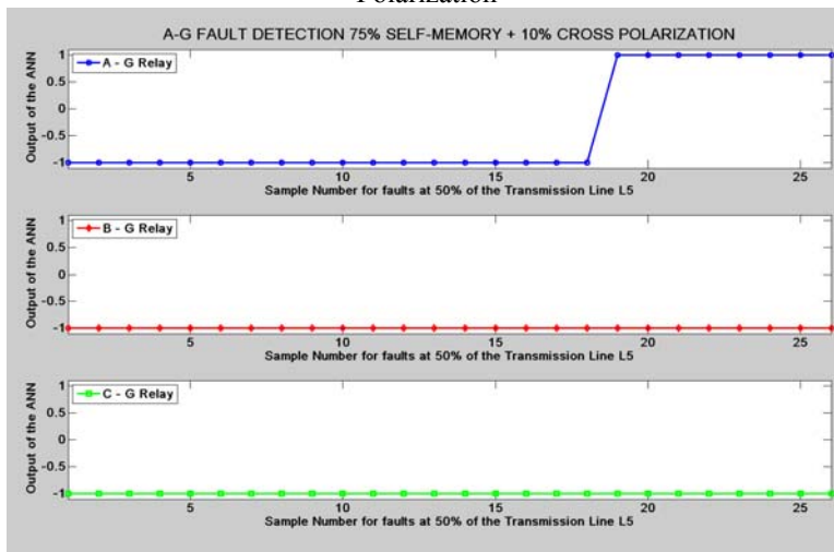
Figure G.187: Mho Relay – SLG Fault at 50% length of L_5 with 75% Self Memory + 10% Cross Polarization
