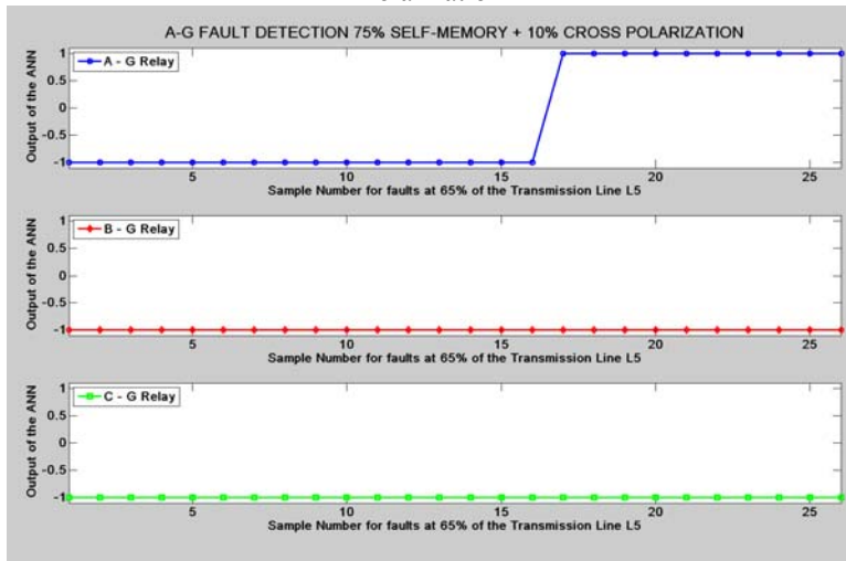
Figure G.190: Mho Relay – SLG Fault at 65% length of L_5 with 75% Self Memory + 10% Cross Polarization
