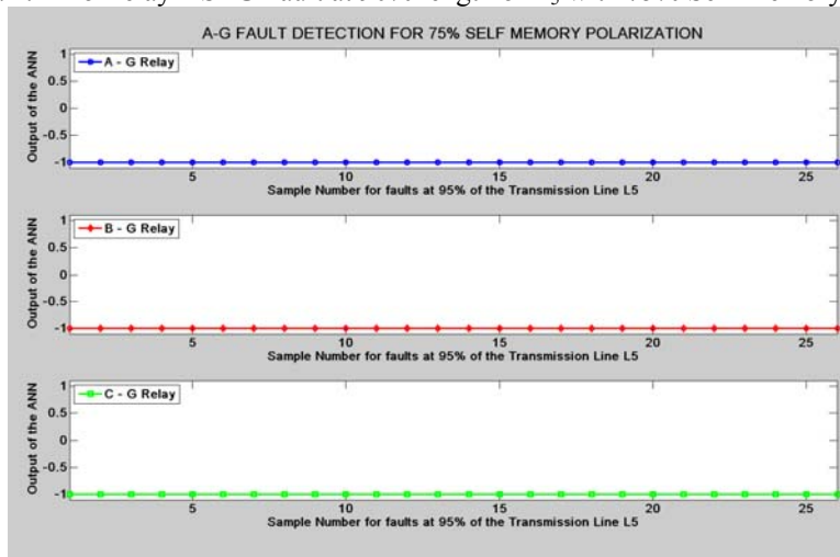
Figure G.175: Mho Relay – SLG Fault at 95% length of L_5 with 75% Self Memory Polarization
