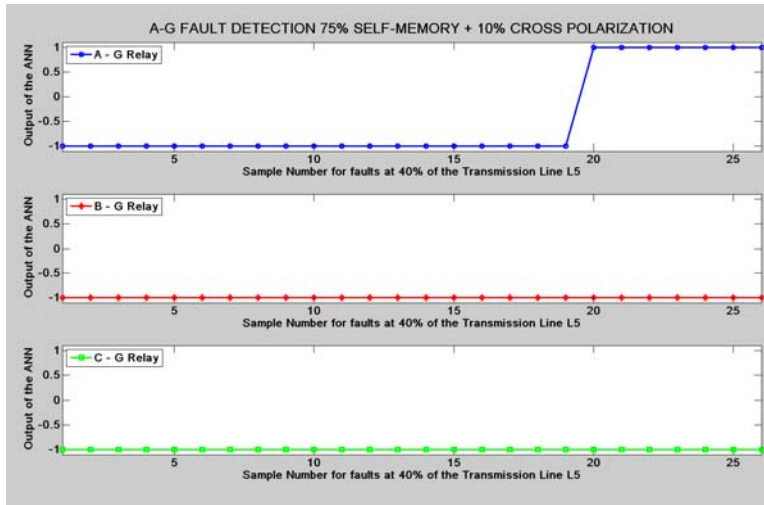
Figure G.185: Mho Relay – SLG Fault at 40% length of L_5 with 75% Self Memory + 10% Cross Polarization
