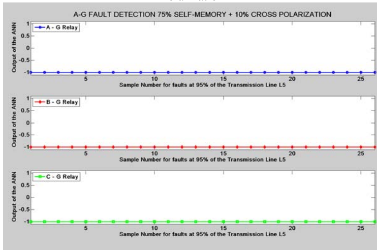
Figure G.199: Mho Relay – SLG Fault at 95% length of L_5 with 75% Self Memory + 10% Cross Polarization
