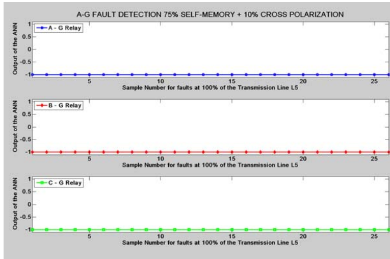
Figure G.200: Mho Relay – SLG Fault at 100% length of L_5 with 75% Self Memory + 10% Cross Polarization
