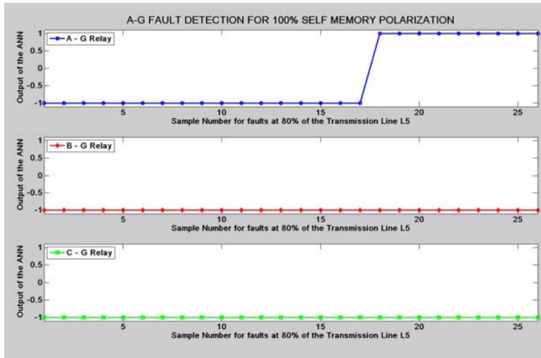
Figure G.146: Mho Relay – SLG Fault at 80% length of L_5 with 100% Self Memory Polarization
