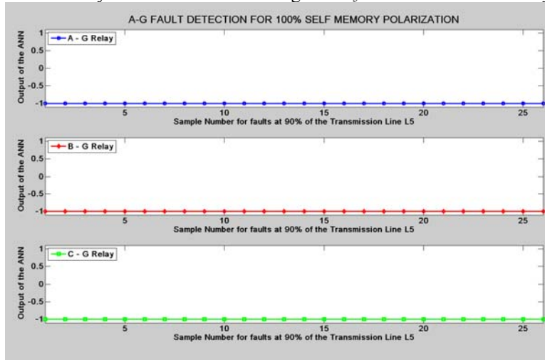
Figure G.150: Mho Relay – SLG Fault at 90% length of L_5 with 100% Self Memory Polarization
