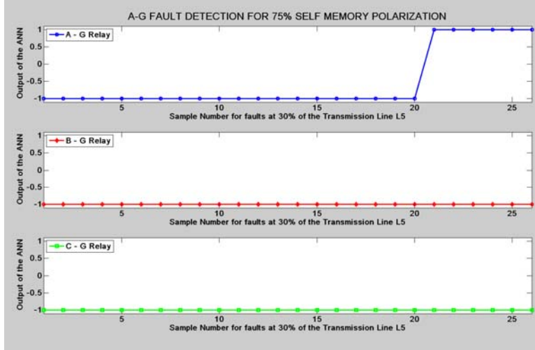
Figure G.159: Mho Relay – SLG Fault at 30% length of L_5 with 75% Self Memory Polarization
