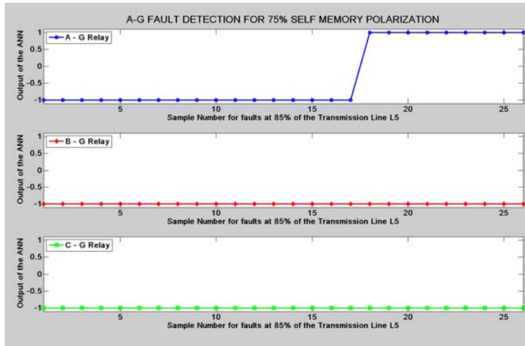
Figure G.173: Mho Relay – SLG Fault at 85% length of L_5 with 75% Self Memory Polarization
