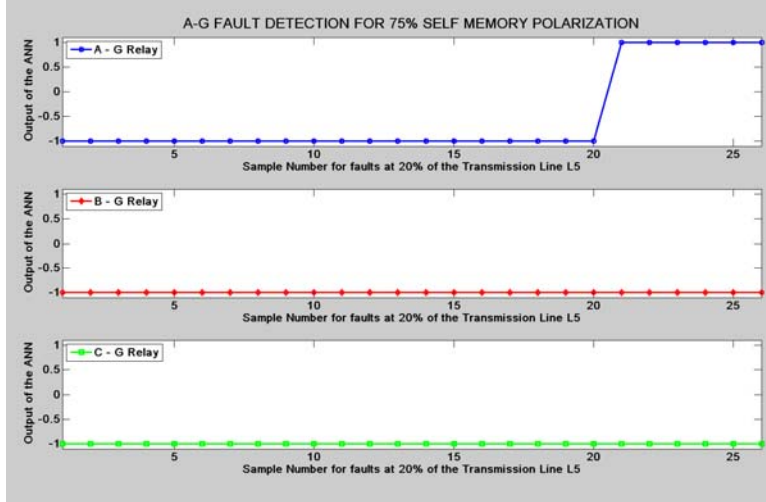
Figure G.157: Mho Relay – SLG Fault at 20% length of L_5 with 75% Self Memory Polarization
