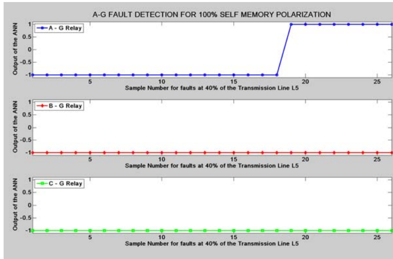
Figure G.137: Mho Relay – SLG Fault at 40% length of L_5 with 100% Self Memory Polarization
