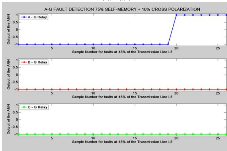
Figure G.186: Mho Relay – SLG Fault at 45% length of L_5 with 75% Self Memory + 10% Cross Polarization
