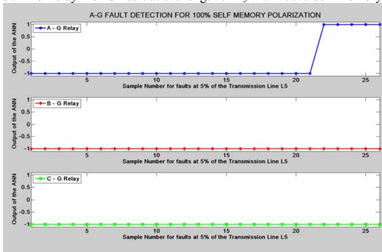
Figure G.130: Mho Relay – SLG Fault at 5% length of L_5 with 100% Self Memory Polarization
