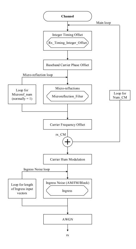
Figure 3.4: Channel Function Flow Diagram
