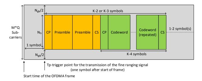
Figure 2.4: Fine Ranging OFDMA Frame Structure [12]
