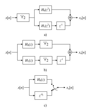
Figure 4.8: Multirate Halfband Upsampler
