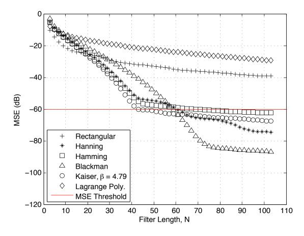
Figure 4.12: Main Path: Worst Case MSE ( $\Delta = 0.5$  samples) vs. Odd Filter Length, No Upsampling
