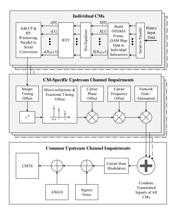
Figure 1.2: Transmitter and Channel System Block Diagram
