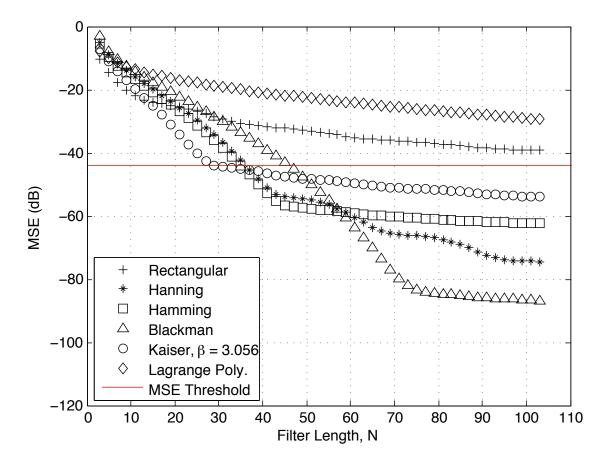
Figure 4.15: Secondary Path: Worst Case MSE ( $\Delta = 0.5$  samples) vs. Odd Filter Length, No Upsampling
