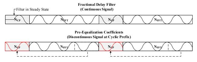
Figure 2.10: Trade-off Between Simulating Micro-reflections Using Fractional Delay Filter vs. Pre-Equalization Coefficients
