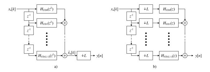
Figure 4.6: Inefficient (a) vs. Efficient (b) Structures for Inducing a Fractional Delay and Performing Decimation
