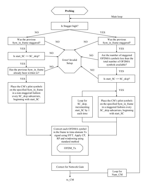
Figure 3.3: Probing Sub-Function Flow Diagram
