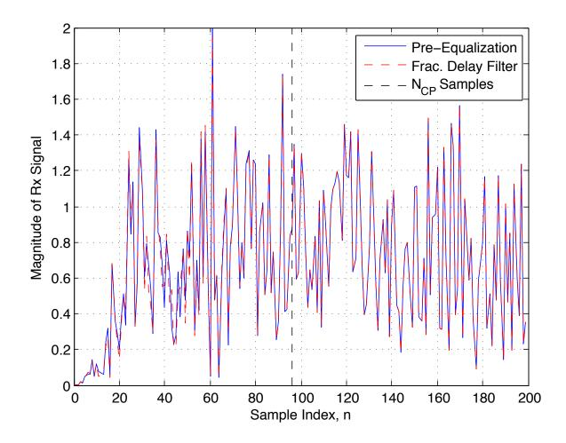
Figure 3.8: Micro-Reflection Verification: Pre-equalization Coefficient Simulation Method vs. Fractional Delay Filter Simulation Method
