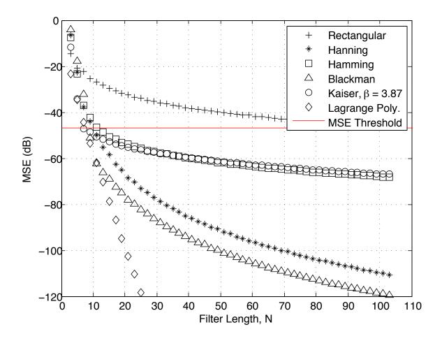
Figure 4.16: Secondary Path: Worst Case MSE ( $\Delta = 0.5$  samples) vs. Odd Filter Length, Signal Upsampled by L = 2
