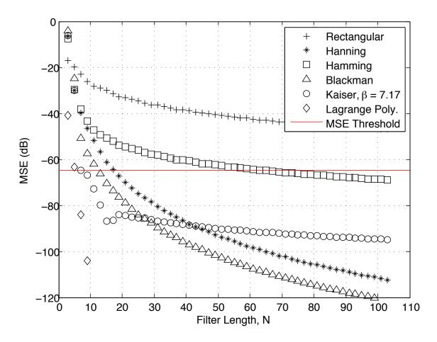
Figure 4.14: Main Path: Worst Case MSE ( $\Delta = 0.5$  samples) vs. Odd Filter Length, Signal Upsampled by L = 4
