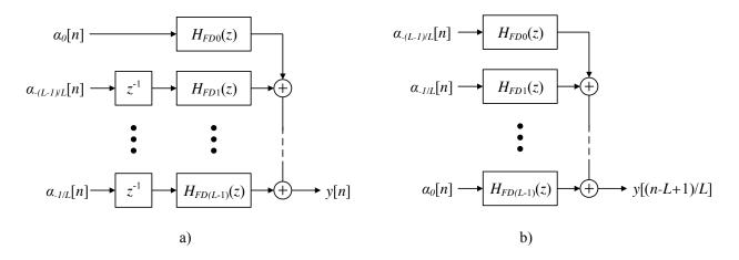
**Figure 4.10:** Connection Sequences Required to Obtain Streams a)  $\alpha_0[n]$  and b)  $\alpha_{-(L-1)}[n]$  at the Structure Output
