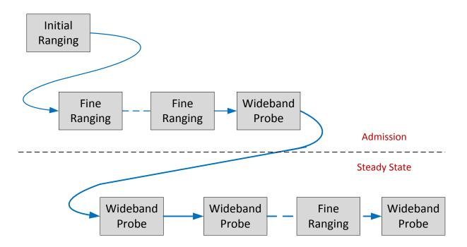
Figure 2.3: Ranging Stages of a DOCSIS 3.1 System [12](c) Cable Television Laboratories, Inc. 2014. Used with permission.
