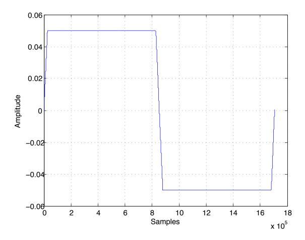
Figure 3.6: 60 Hz Carrier Hum Waveform,  $F_s = 102.4$  MHz
