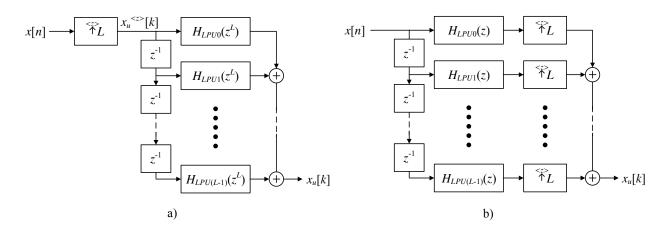
Figure 4.5: Inefficient (a) vs. Efficient (b) Structures for Performing Interpolation
