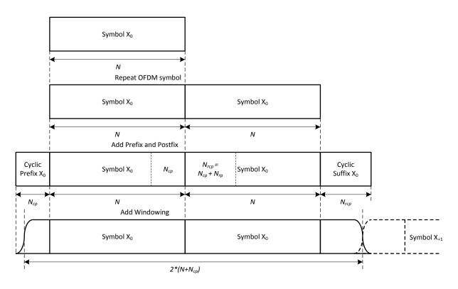
Figure 2.5: Fine Ranging OFDMA Symbol Structure [12](c) Cable Television Laboratories, Inc. 2014. Used with permission.
