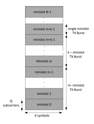
Figure 2.1: General OFDMA Frame Structure with Minislots [12] © Cable Television Laboratories, Inc. 2014. Used with permission.
