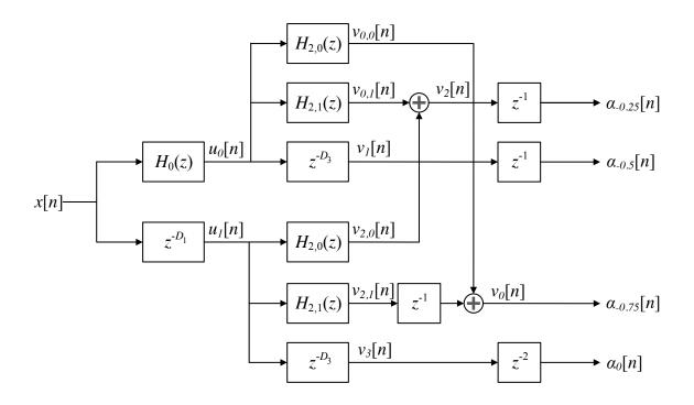
Figure B.1: Single-Sampling-Rate FIR Halfband Cascade, L = 4
