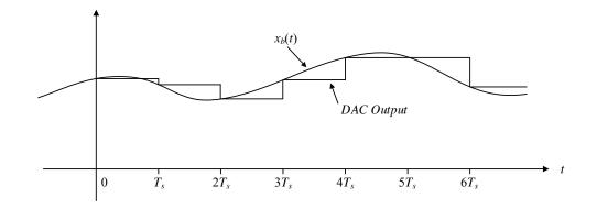
Figure 2.7: Sample and Hold DAC Output vs. Reconstructed Signal
