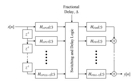
Figure 4.11: Single-Sampling-Rate Structure with Delay and Switching Logic
