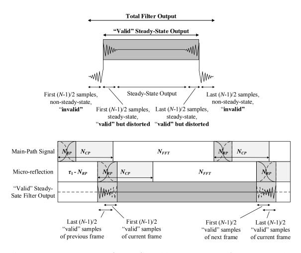
Figure 3.5: Distorted Filter Output Caused by Using Frames of a Finite Length to Simulate Micro-reflections
