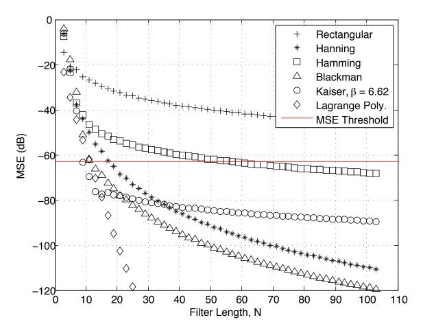
Figure 4.13: Main Path: Worst Case MSE ( $\Delta = 0.5$  samples) vs. Odd Filter Length, Signal Upsampled by L = 2
