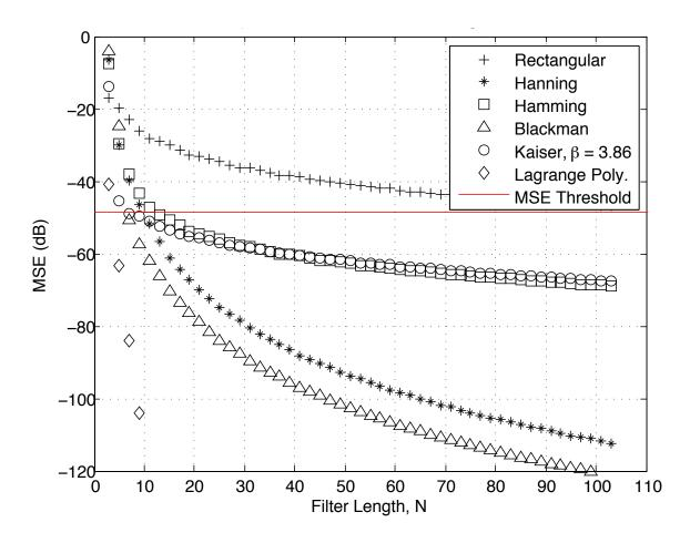
Figure 4.17: Secondary Path: Worst Case MSE ( $\Delta = 0.5$  samples) vs. Odd Filter Length, Signal Upsampled by L = 4
