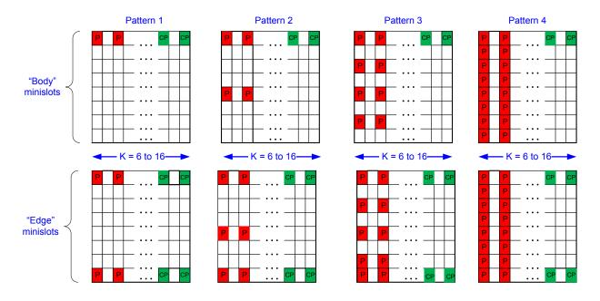
Figure 2.2: Pilot Patterns 1-4, 2k Mode [12]© Cable Television Laboratories, Inc. 2014. Used with permission.
