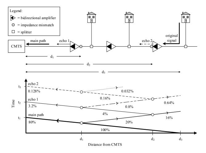
Figure 2.9: Example of Micro-reflections in an HFC Network
