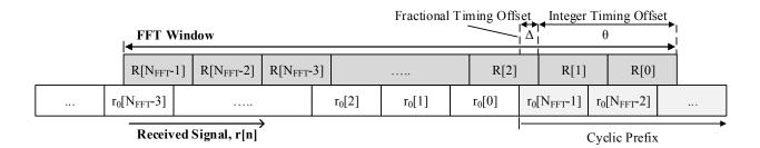
Figure 2.8: Timing Offset of a Received OFDMA Frame
