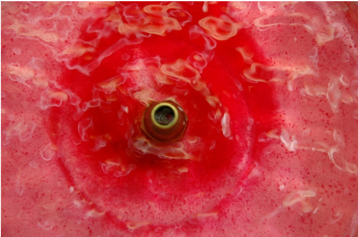
(a) Raw image of vibrating system with a solid obstacle (infinite impedance).
