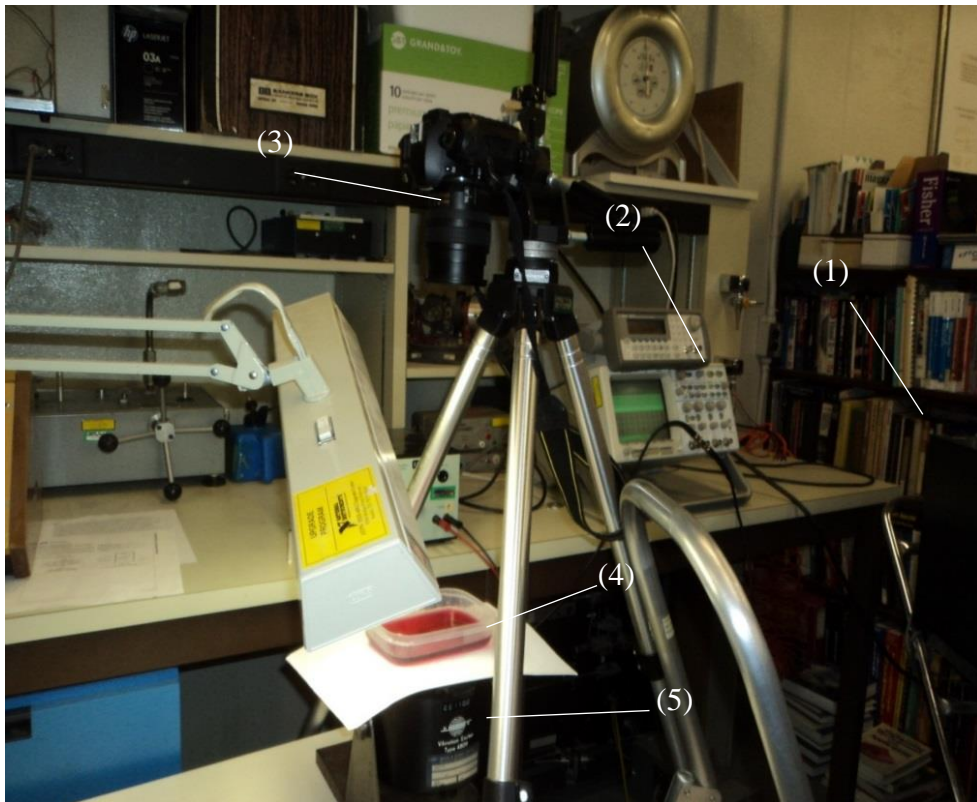
Figure 3.1: Experimental setup for liquid vibrating system, (1) Dual channel analyzer, (2) Oscilloscope, (3) Digital Camera, (4) Liquid container, (5) Multi-vibration exciter
