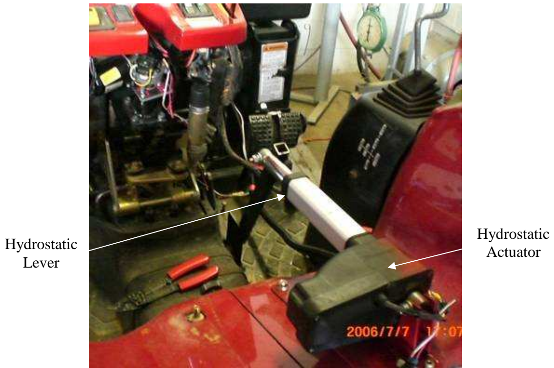
Figure 4.2: The tractor with the seat removed and the hydrostatic DC actuator installed
