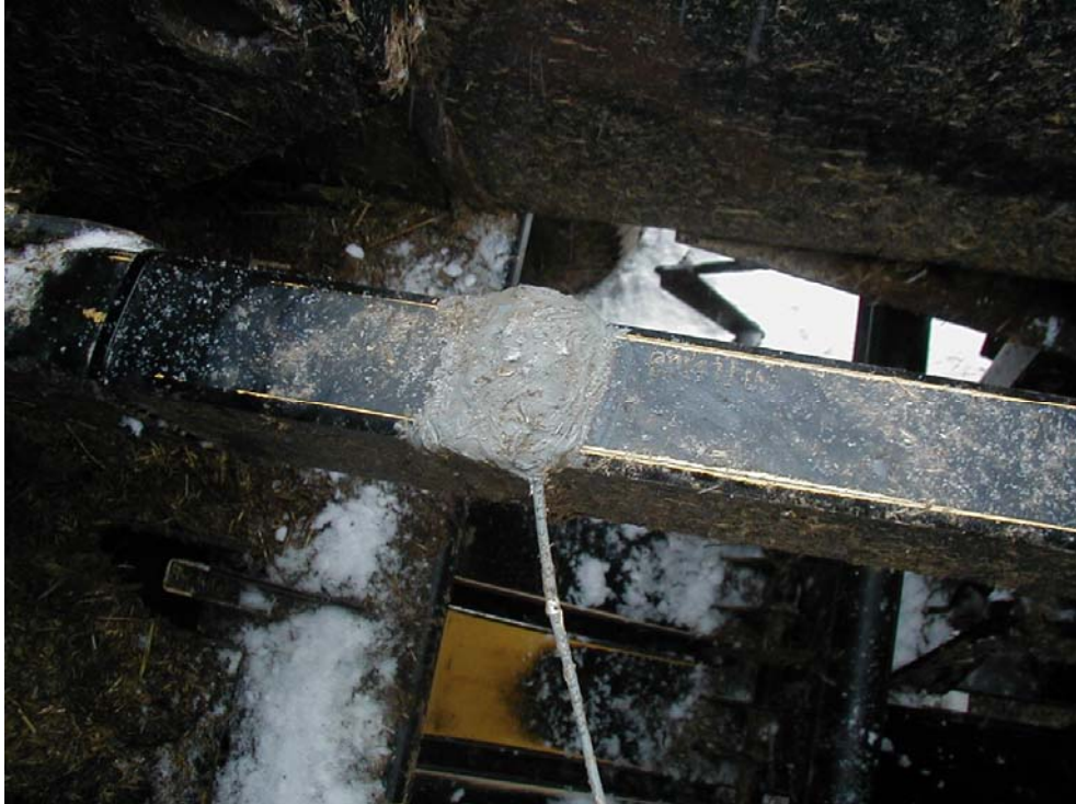
Figure 3.14 Strain gages installed on the plunger arm.
