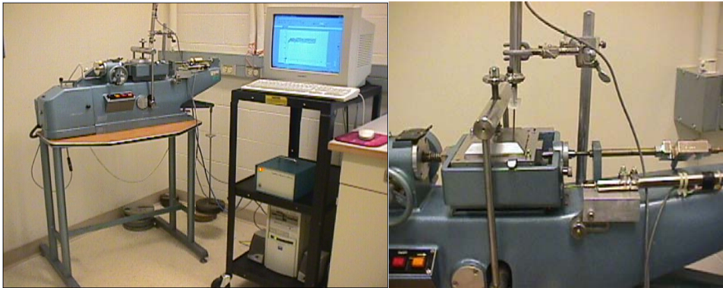
Figure 3.38 Measurement of the coefficient of friction using Wykeham Farrance shear box.
