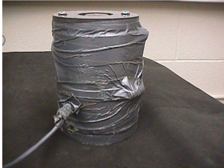
Figure 3.17 Assembled uni-axial sensor (height is 150 mm).
