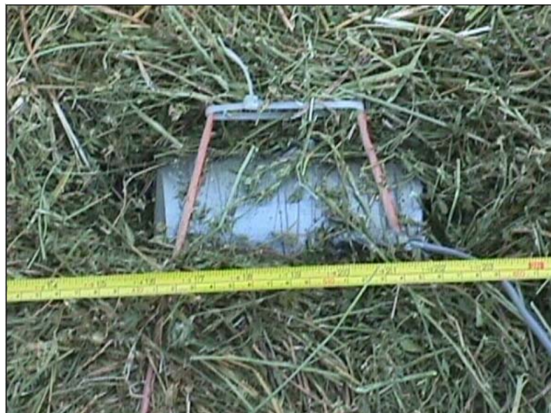
Figure 3.33 Load cell inside the bale in the z -direction.
