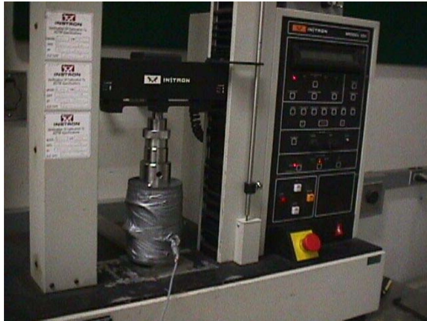
Figure 3.18 Load cell calibration using the Instron testing machine.
