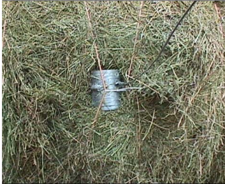
Figure 3.34 Load cell inside the bale in the y -direction.
