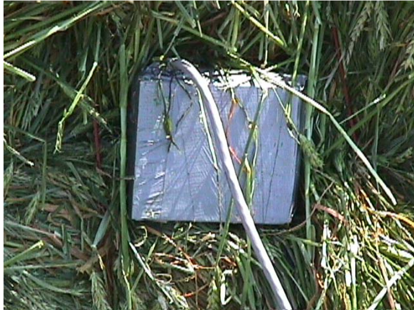
Figure 3.36 Tri-axial sensor inside the whole green barley bale.
