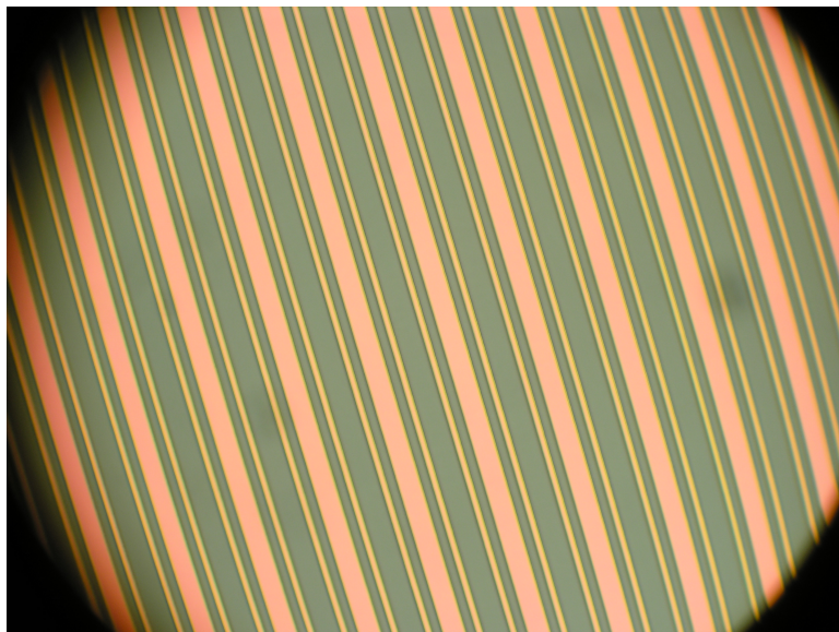
Figure 2.1: Optical image of acrylic template used to form PDMS stamps (image size 326.4 \times 244.8 \mu\text{m} )
