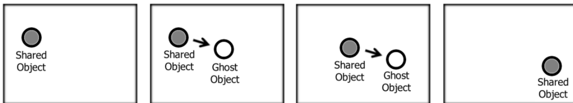
Figure 2.4. The ball is being moved across the screen by the user. In the Echo technique, the ghost object represents immediate feedback while the shared object is updated from the network.
