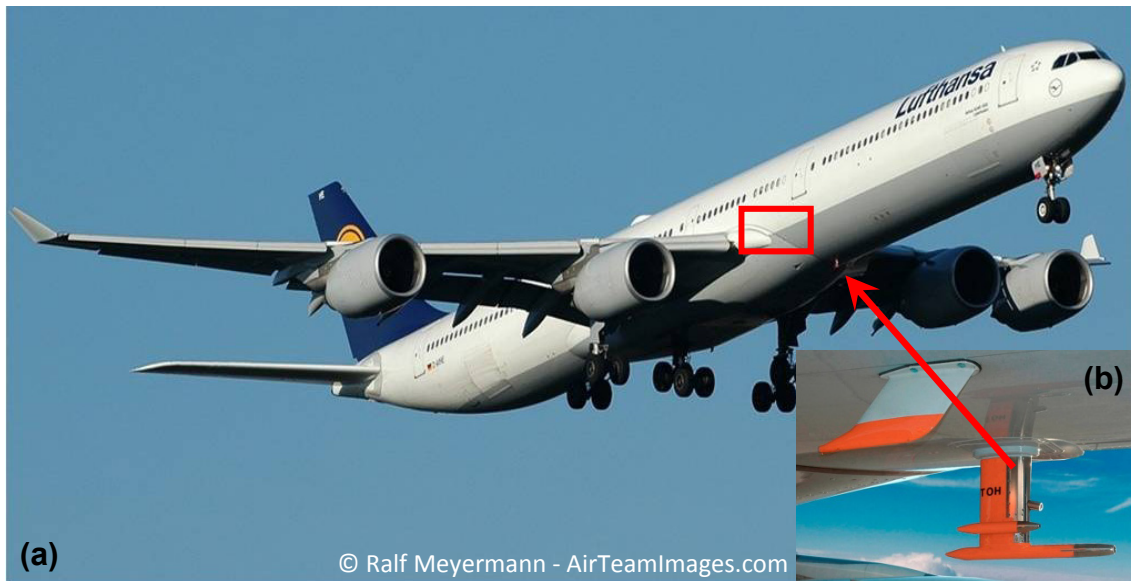
Figure 3.2: The CARIBIC aircraft with the gas and aerosol inlet. Figure (a) shows the aircraft, the Airbus A340-600 “Leverkusen” (D-AIHE) from the German Lufthansa AG. The arrow marks the position of the inlet, and the red box the position of the measurement container inside the forward cargo bay. Figure (b) shows the permanently mounted inlet, which is located about 23 m behind the nose of the aircraft.
