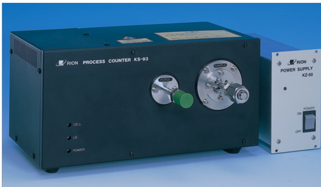
Figure 4.3: Optical Particle Counter KS-93 (RION) with power supply KZ-50 (from www.rion.co.jp/english/ ; last access: 20.07.2014).
