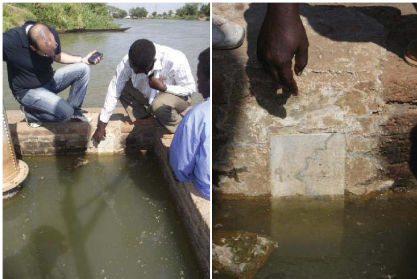
Figure 2-8. Measuring the water level to estimate the daily discharge of the Gezira channel during the field visit (26/12/2011)
