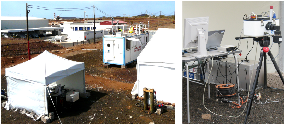
(a) FTIR tent (lower left) and LIDAR container with radiometric instrumentation on top (b) D&P Model 102 without sun-shield
