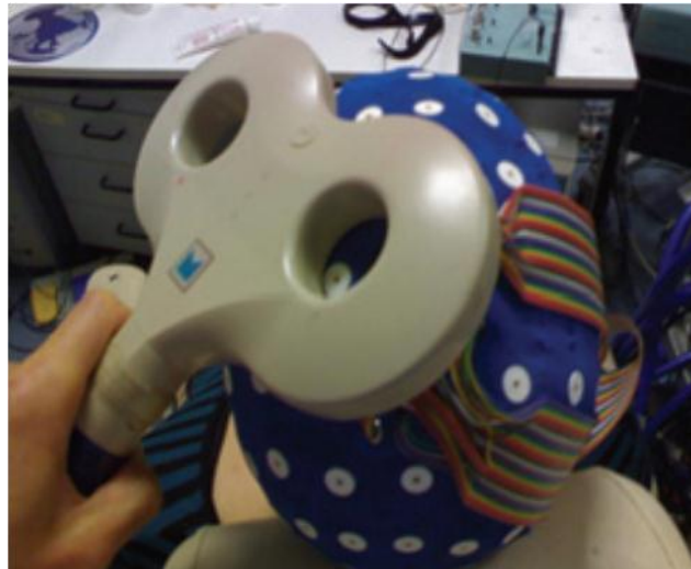
Figure 4: Illustration of combined method of TMS and EEG
